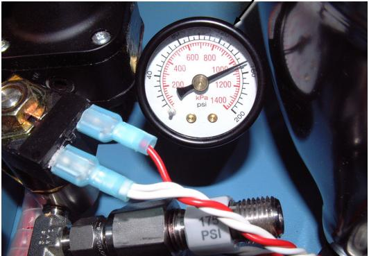
2500 internal pressure gauge/regulator adjustment should be set between 145-150 psi. Note: The 2500 system must be in the run mode.
