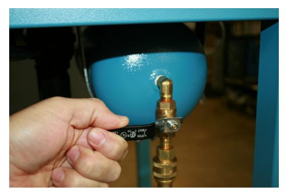
3. Remove the air supply line from the back of the system using a 9/16" wrench.
