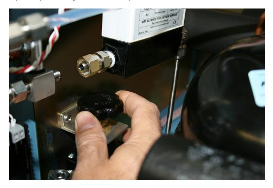
20. Put a thumb over the exposed flow meter fitting.
