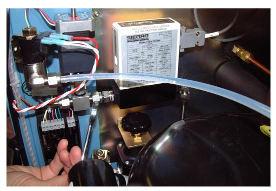
9. Remove the nut at the base of the regulator outlet using a 9/16" wrench.
