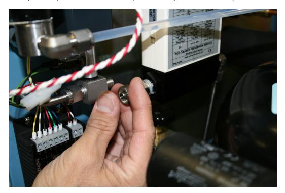
22. Block and release with your thumb several times until the flow meter is dry, and you begin to get actual readings of flow on the front screen again.
