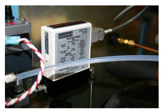
8. Remove the nut on the air outlet side of the flow meter using a 9/16" wrench.
