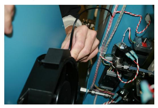
7. Locate the flow meter on the inner wall of the cabinet.
