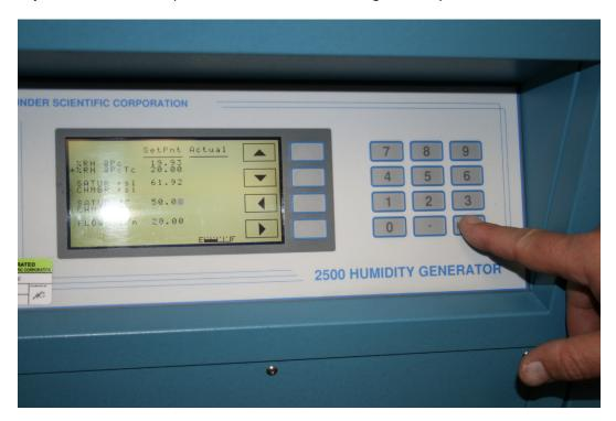
18. Press the RUN key to start the generator. This will activate the air supply solenoid.
