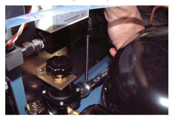
10. After unscrewing the two nuts, rotate the flow meter slightly clockwise.
