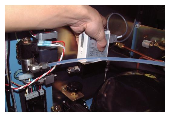
11. Reinstall the flow meter only using the lower nut at the regulator outlet and leave the other exposed.
