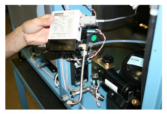
7. Next remove the two screws of the data cable using a small flat head screwdriver.
