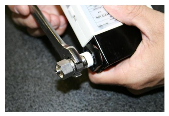
13. Make sure that the air in tube is parallel to the body of the flow meter.
