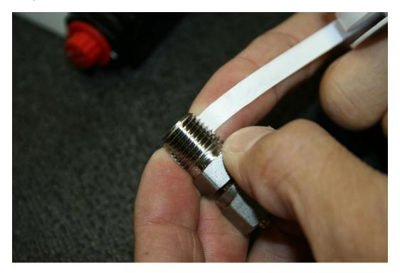
12. Insert the stainless steel air in and air out fittings into the plastic fittings and make sure not to over tighten them. Leave about three to four threads showing.
