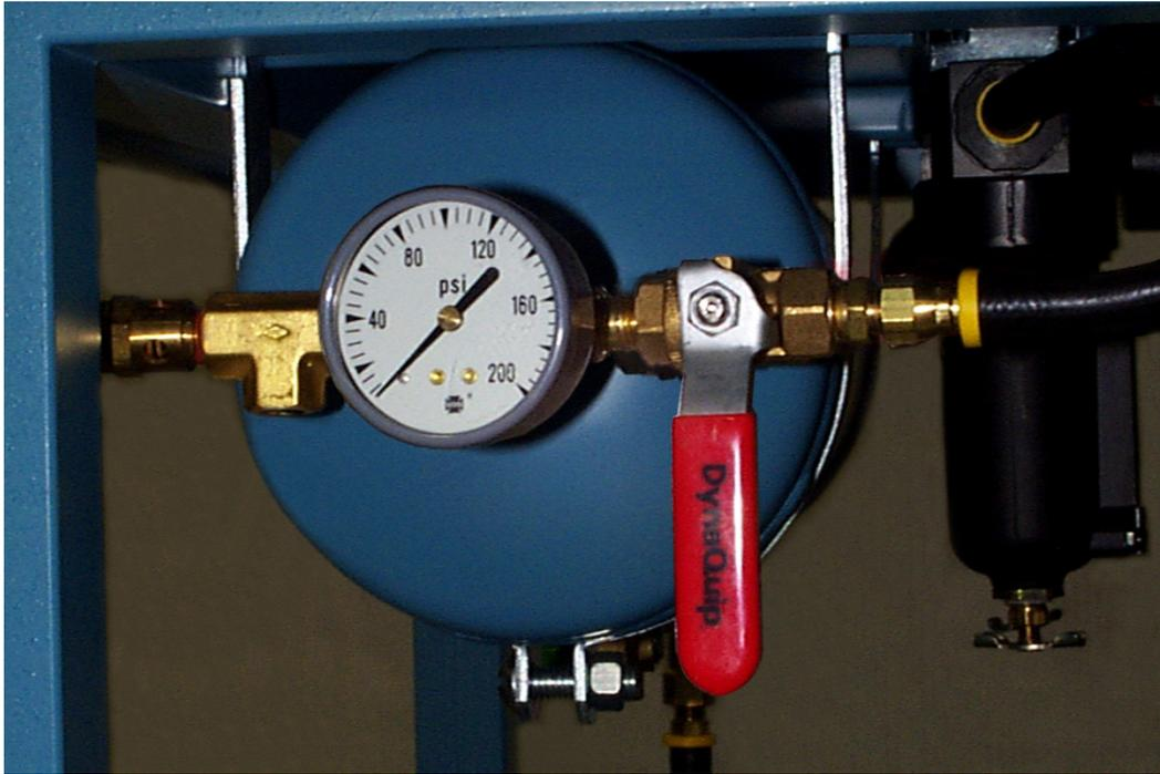
8. Insert the adjustable relief valve in the bottom opening of the tee. The adjustable valve has been preset at 175 psiG.
