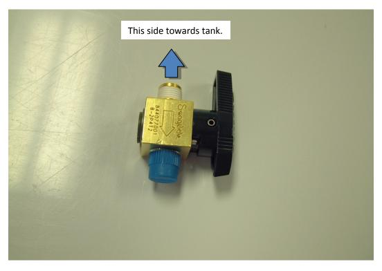
6. Use a 3/4" open end wrench to install the drain valve. Make sure the handle of the valve faces the handle of the cart. Note: the air tank you have may not look the same as pictured.
