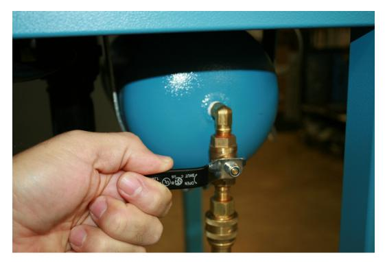
3. Turn the air tank drain valve to the open position to bleed off any excess air, be sure to hold a rag underneath the drain to catch any small amount of water that may release.
