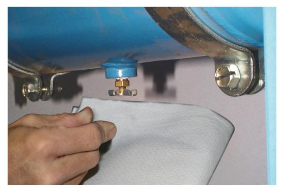
4. Remove the drain from the air tank using a 7/16" wrench.
