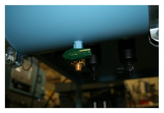
8. Next open the air tank input valve.
