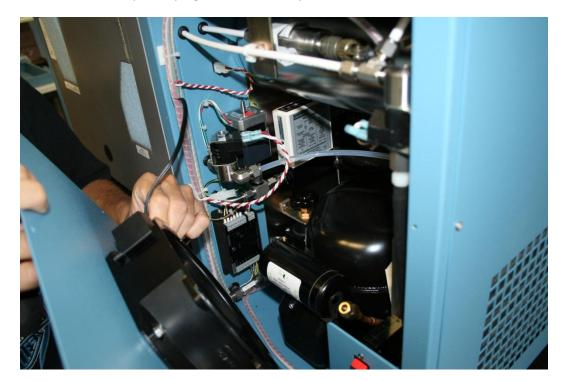
2. Remove the right rear panel and disconnect the exhaust fan power connection.
