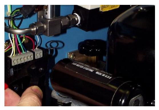
16. Replace the right rear panel and the exhaust fan power connection.
