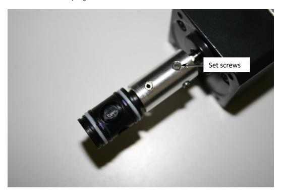
8. Remove the value plug from the value body and remove the O-Rings. You may have ether the plug on the right or left, replace only the ones that came with your system.
