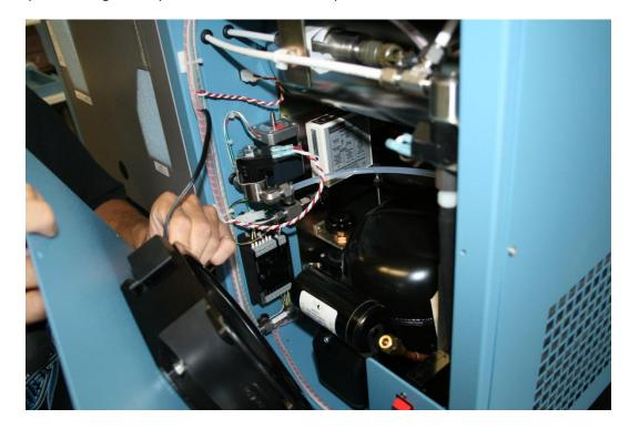
17. Replace the Torx head screws on the right rear panel and connect the main power cord as well as air in connection to the elbow.
