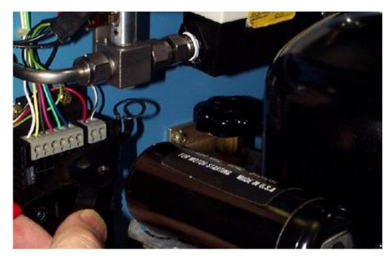
3. Remove the snap ring at the base of flow valve.
