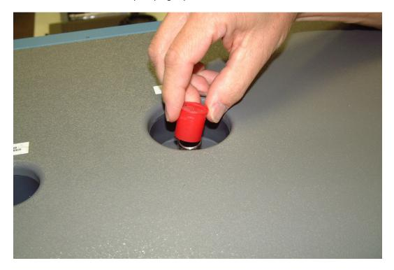
8. Use a funnel that will fit into a 5/8" (15.9mm) diameter opening.
