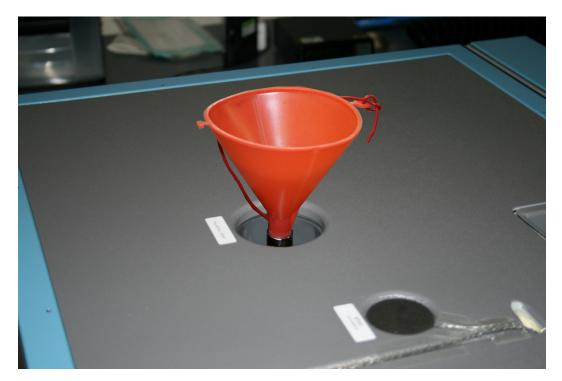
9. Using 3 U.S. gallons of -100 °C propylene glycol fluid (4 U.S. gallons for 2500ST models), fill until unit level is approximately 1/4" (6.35mm) below the bottom of the fill port.
