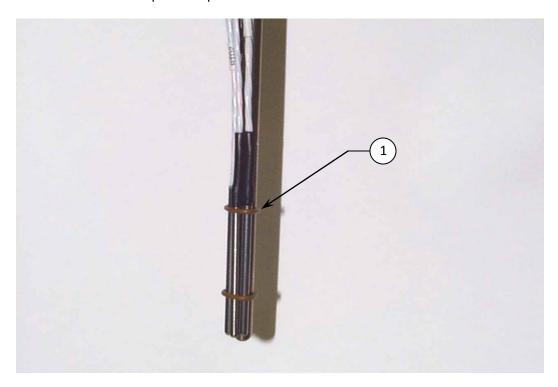
3. Take item (2) rubber sheath, and slide it over the probes and the thermometer.
