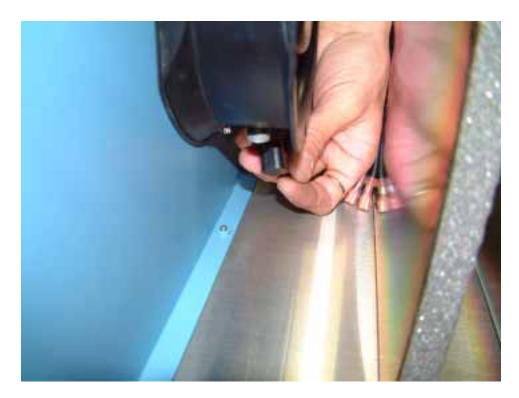
46) Connect the two black wire terminal connectors to the hour meter terminals.
