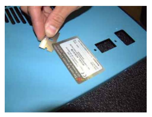
Take great care when lifting off the label so that no damage occurs because you will reuse the label on the new panel.
