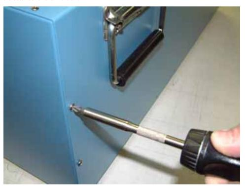
2) Loosen the electrical bulkhead fitting.
