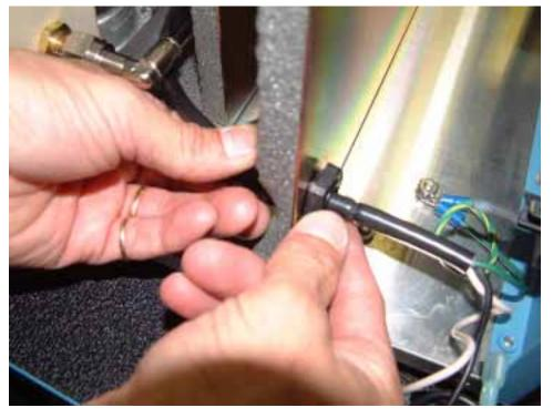
41) Reconnect the red line to the plug receptacle terminal to the rear and connect the compressor/fan harness to the front plug receptacle terminal.
