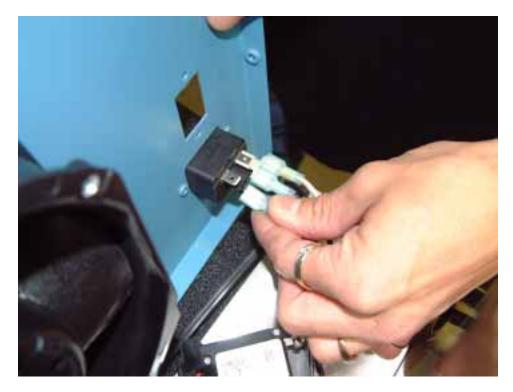
10) Remove the top right dual terminal connector from the electrical power cable receptacle.
