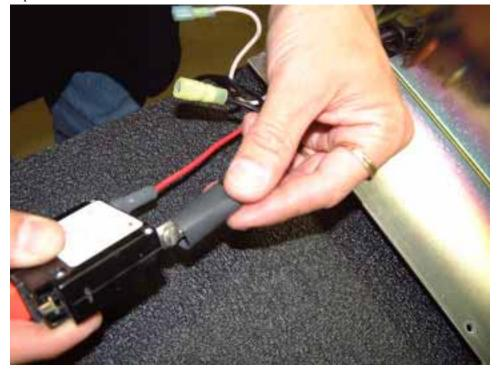
Take the white wire from the compressor and the black from the fan/hour meter harness and slide the multi-stack adapter inside each terminal connector..
