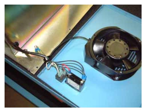
6) Disconnect the exhaust fan power connection.
