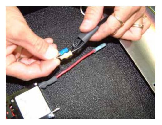
32) Set the two terminal rings over the top screw tab of the power switch.
