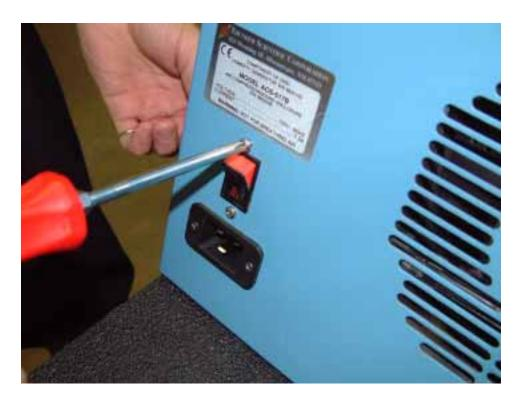
8) Remove the 4-40 screws from the electrical power cable receptacle.
