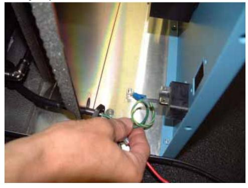
39) Use the existing hardware to hold the terminal rings down.
