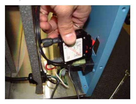
44) Use the same screws to mount the power switch.
