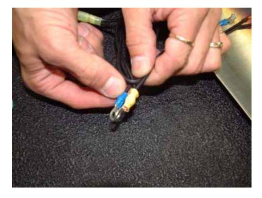
31) Next slide the heat shrink tubing that was provided over the terminal rings.
