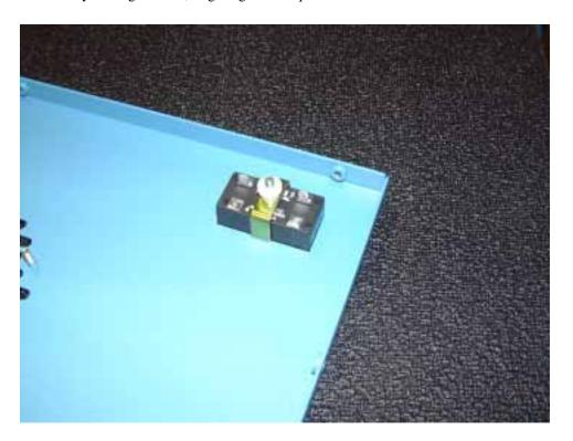
24) Replace the nylon washers you removed from the old panel for the fan.
