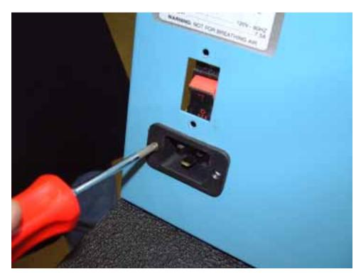
9) Remove the top left terminal connector from the electrical power cable receptacle.
