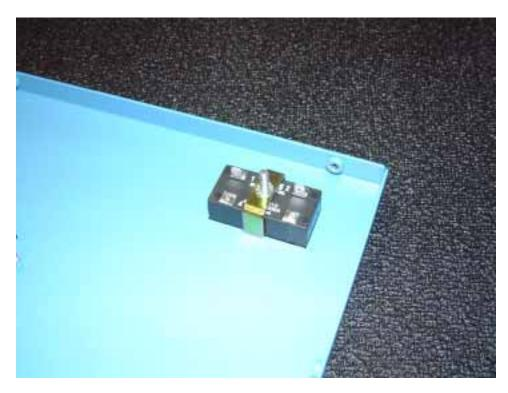
23) Twist on nylon finger screw, finger tight is adequate.
