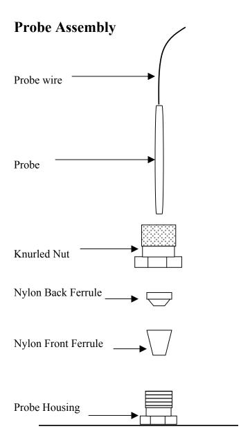
Note: ferrules must retain Probe. Do not use wire to retain.
