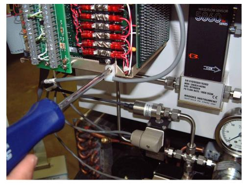
4) The machine needs to be reset for the new transducer as follows. First plug in the system and power it up. On the main screen press the EDIT/CAL option button.
