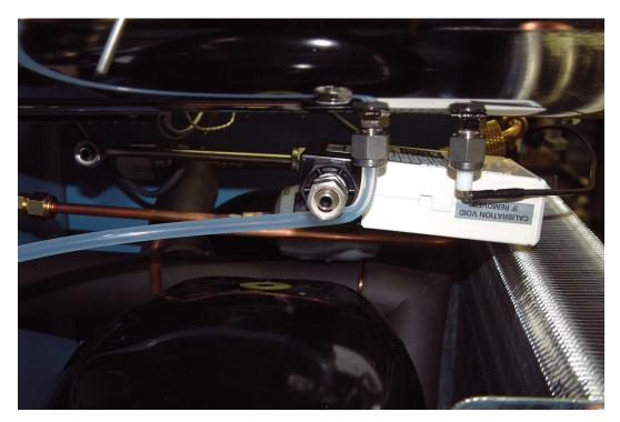
12. Using a flat head screwdriver, pry the wire leads off of the solenoid valve.
