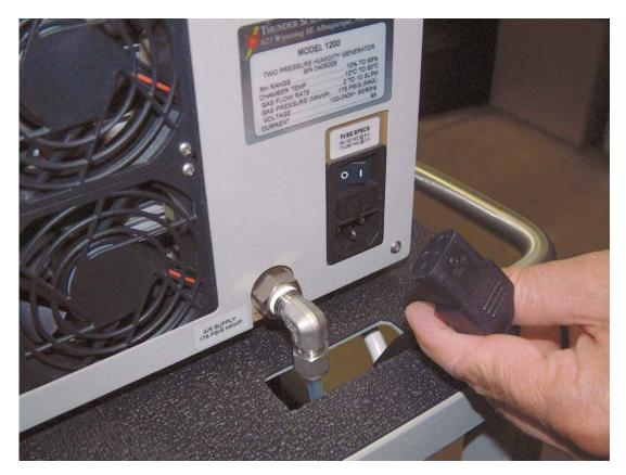
1. Remove power cord and disconnect air in line.
