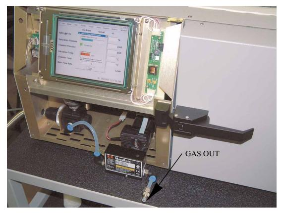
9. Gas is now flowing through the regulator and flowmeter. Apply thumb over the tubing as shown. Allow the 1200 to pressurize to 30 psiG, then release.
