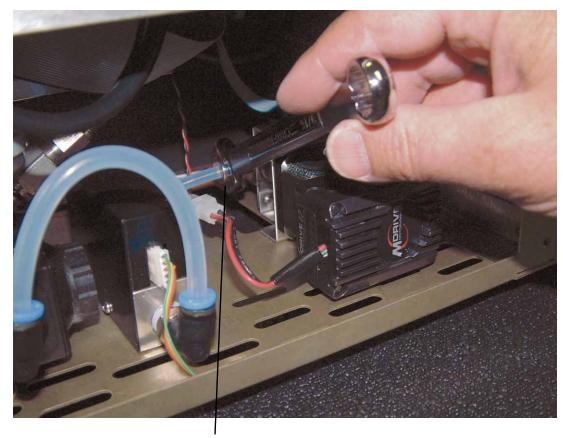
4. Disconnect tubing at the flow control valve inlet.
