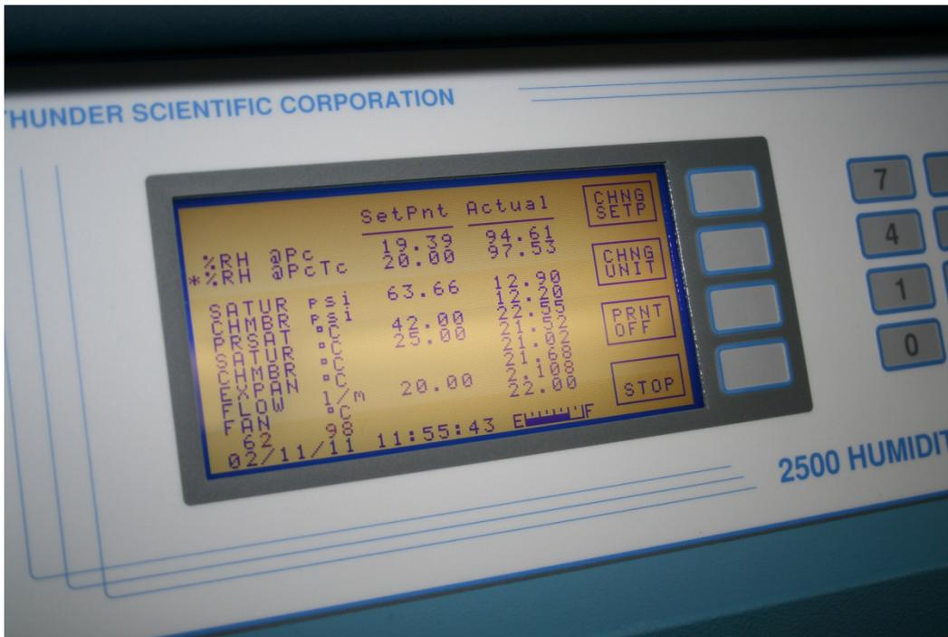
Pre-Sat heat delta should be +15 deg above saturation temperature set-point; expansion valve heat delta should be 1-1.5 deg above chamber temperature actual.
