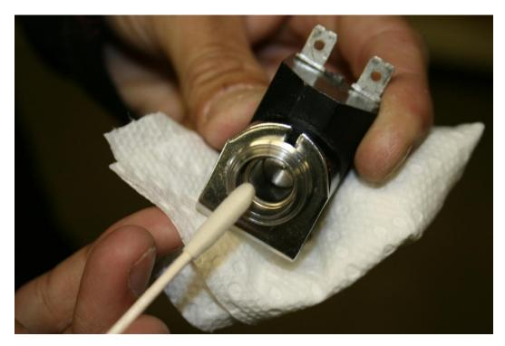
19. Replace the o-ring in the valve body making sure it's properly seated.
