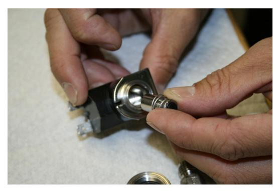
21. Put the coil housing and the valve body together.
