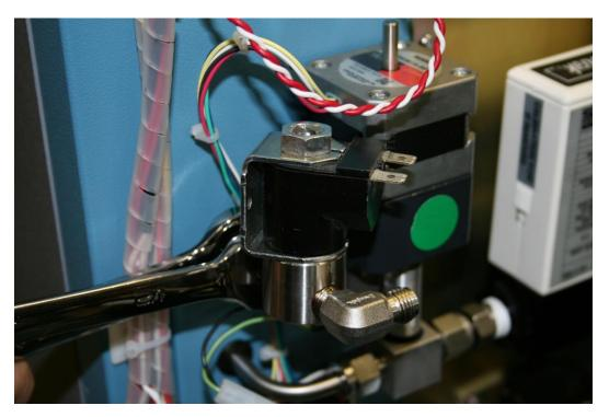
8. Take the solenoid to a workbench and clamp the stainless steel body in a vice.
