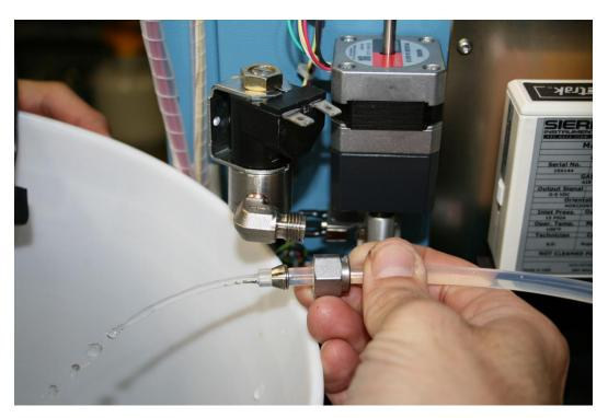
7. Remove the pre-sat fill solenoid using a 9/16 wrench and a 1/2 wrench.
