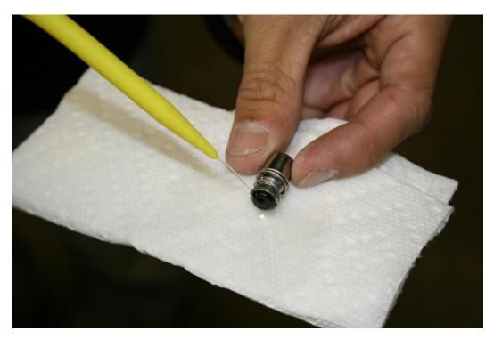
15. Clean the valve body with alcohol.
