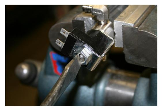
9. Using a flat head screwdriver, unscrew the coil from the body.
