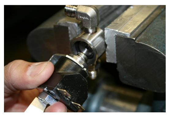
11. Take out the coil plug and spring from the coil housing.
