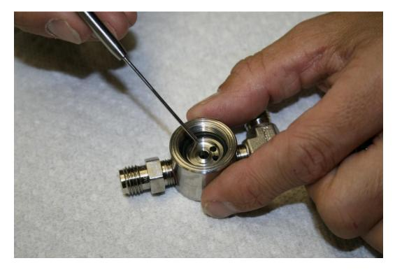
20. Next insert the coil plug and spring inside the coil chamber housing.
