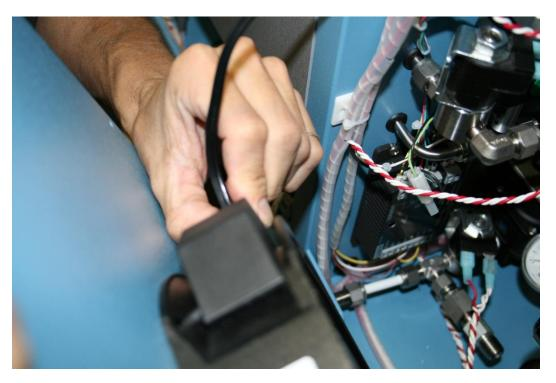
4. Locate the Pre-Sat fill solenoid and remove the wire leads using a small flat head screwdriver.
