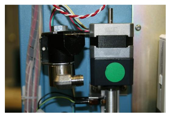
25. Reattach the reservoir to pre-sat solenoid tube using a 9/16 wrench and a 1/2 wrench, be sure not to over tighten.
