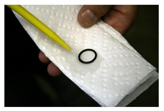
14. Clean the coil plug and spring with alcohol.
