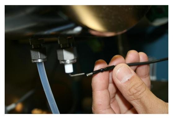
8. Using a flat head screwdriver, slide off the two connections on the pre-sat fill solenoid.
