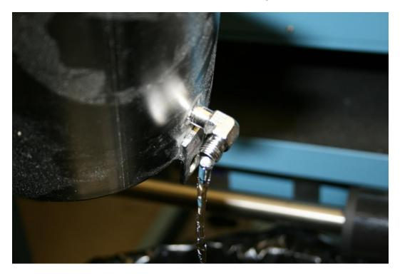
19. Using a 9/16 wrench, remove the reservoir to pre-sat solenoid tube from the reservoir.
