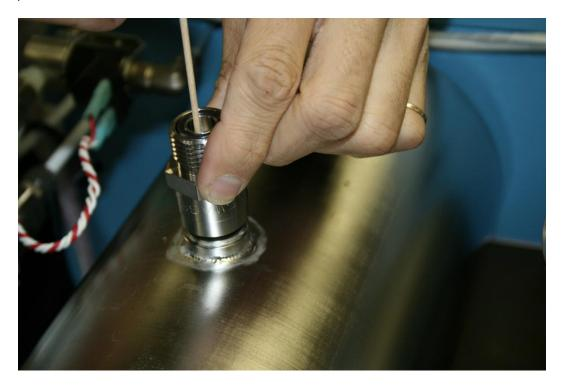
44. Using an adjustable wrench tighten the fill port extension, do not over tighten o-rings are present.
