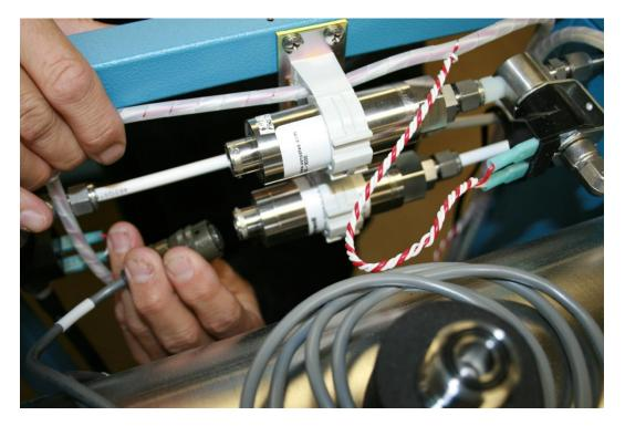
13. Pull back the transducer cables that are coiled on top of the reservoir.
