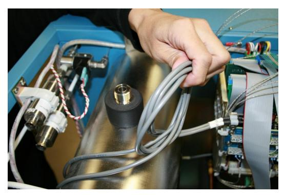
14. Using a 9/16 wrench loosen and pull away from the reservoir, the pressure balance tube.
