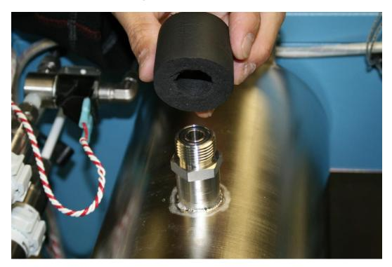
46. Replace the transducer cables and the temperature probe cables coiled over the fill port extension.
