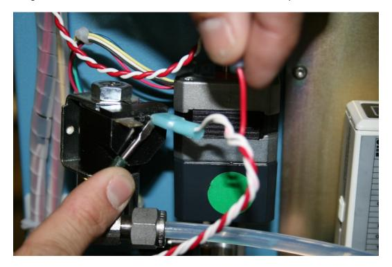
9. Remove the pre-sat fill solenoid using a 9/16 wrench and a 1/2 wrench.
