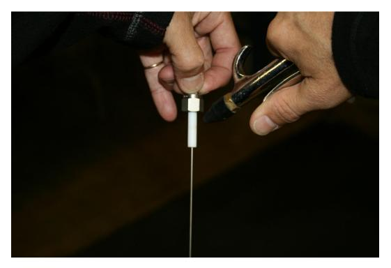
31. Insert the liquid level probe assembly back into the reservoir (See step 20 for precautions) at the fitting on the end.
