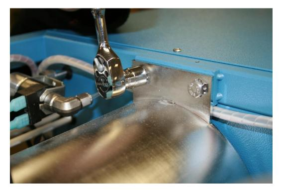
17. Holding both the reservoir and the pre-sat solenoid together, remove all three 7/16 bolts and slide out the reservoir.
