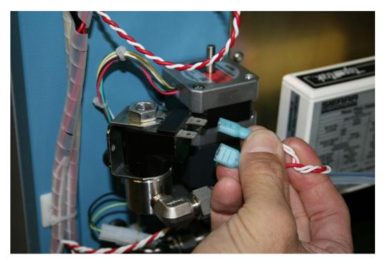
40. Reconnect the liquid level probe indicator cable.
