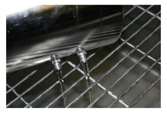
27. Remove the reservoir to pre-sat solenoid tube from the solenoid using a 9/16 wrench.
