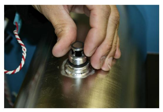
43. Take a long cleaning swab and feed it through the fill port extension and place the swab on the poppet to hold it in place. Then slide the fill port extension over the poppet and screw into place.
