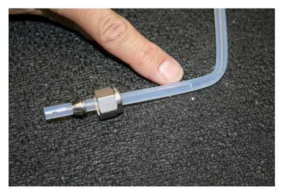
29. Next clean the liquid level probe assembly with alcohol.
