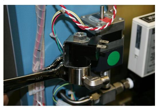
37. Reattach the pre-sat fill solenoid using a 9/16 wrench and a 1/2 wrench making sure that the elbow is level with the frame.
