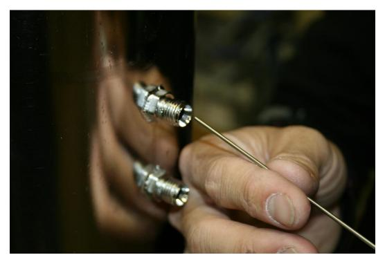
32. Tighten the nut of the liquid level probe assembly, but do not over tighten and make sure the probe lead faces the front of the system.
