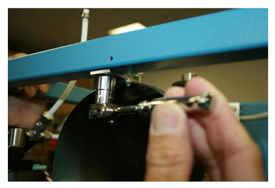
16. Loosen both 7/16 bolts that secure the reservoir to the frame.
