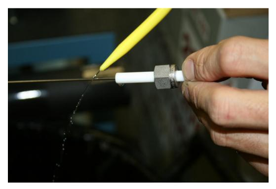
30. Blow dry the liquid level probe assembly.
