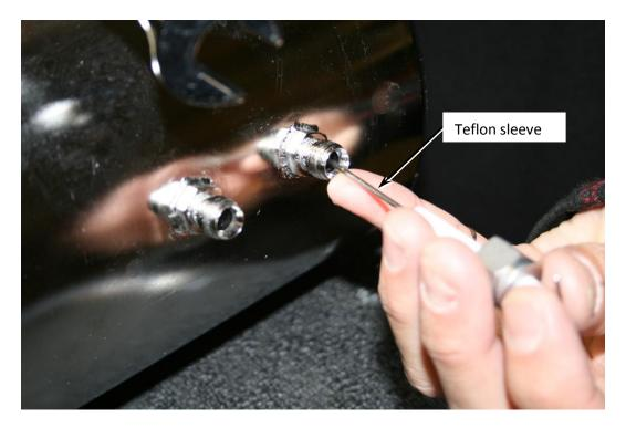
21. Remove the insulation from the reservoir fill port.
