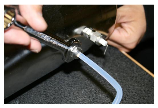
20. Remove the reservoir liquid level probe assembly from the reservoir using a 9/16 wrench. Be careful not to scrape the sides of the probe when removing it, because damage could occur to the Teflon sleeve.
