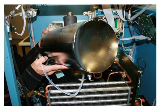
18. Next take the reservoir to a sink or bucket to drain the foreign matter from the reservoir.
