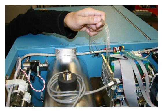
47. Reconnect the transducer cables to T2 and T3.
