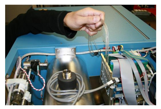
11. Disconnect the transducer data cable (T2).
