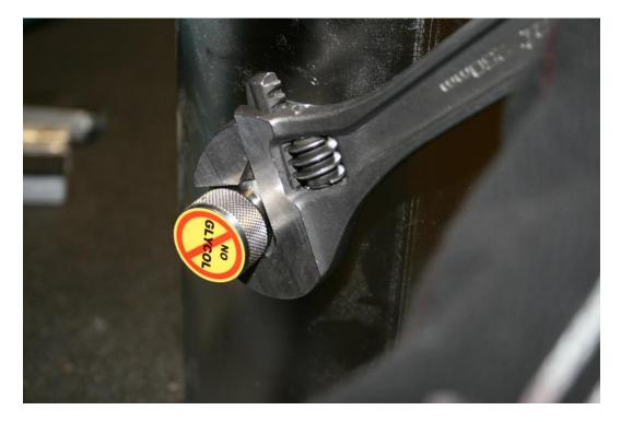
23. At the base of the reservoir fill port assembly there will be some parts that need to be saved.
