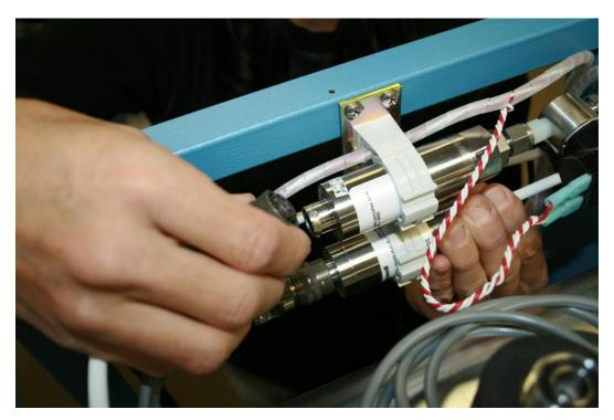
12. Disconnect the transducer data cable (T3).
