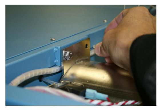
35. Reattach the reservoir to pre-sat solenoid tube, do not over tighten.
