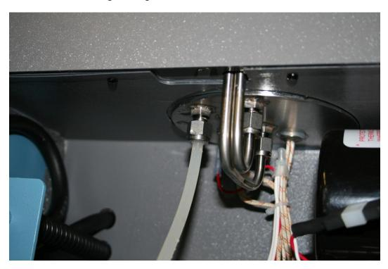
12. Place a one gallon bucket under the tube and let it drain.
