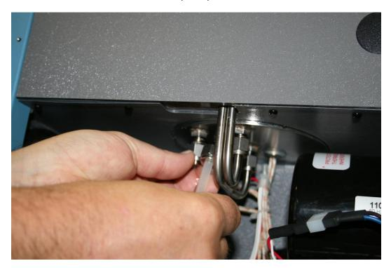
10. Place the tube in close proximity to the Pre-Sat drain nut and swap out the two.
