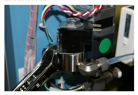
19. Reconnect the wires back to the solenoid.
