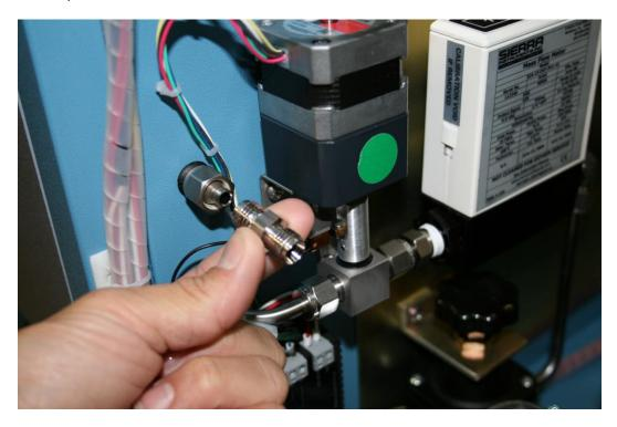
14. Place a hose with a 1/4 tube fitting on the union.
