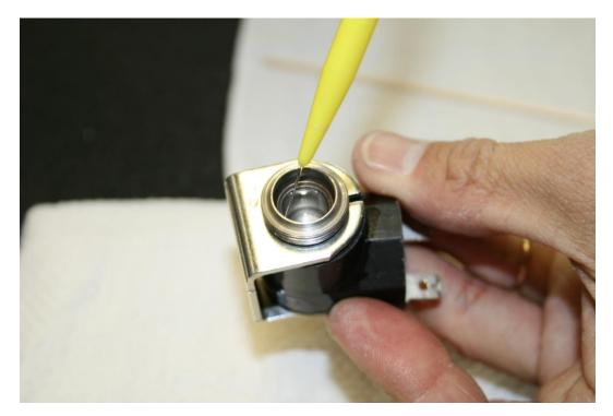
17. Use a swab to get any debris out of the coil housing.
