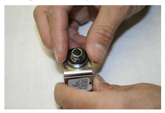
24. Next take a swab with alcohol on it and clean the inside of the valve body still on the frame.
