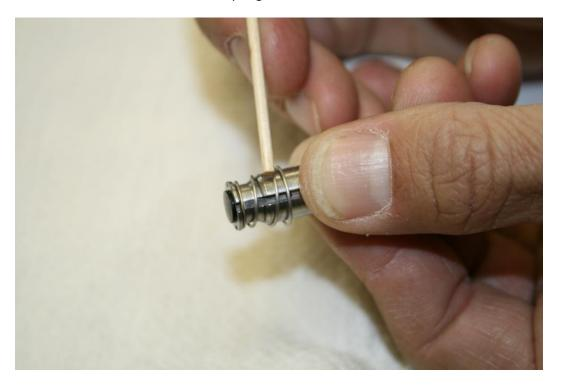
16. Clean inside the coil housing with alcohol.
