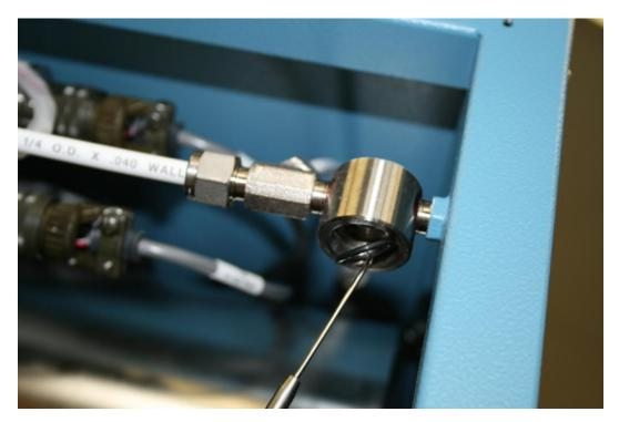
11. Using alcohol, pour some on the valve coil plug and spring from the coil housing.
