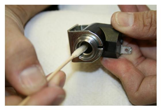
18. Blow out the coil housing and make sure its dry.
