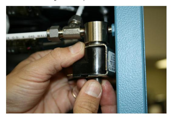
26. Using the large flathead screwdriver from step 8, tighten until snug.
