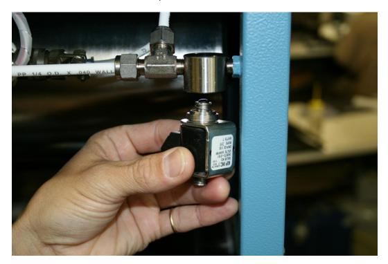
10. Inside the valve body is an o-ring, remove it carefully.
