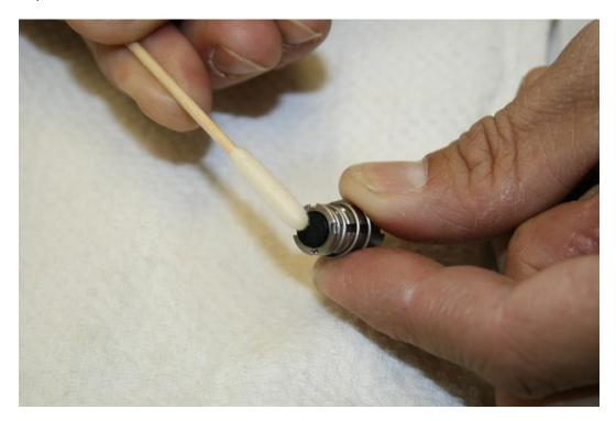
13. Clean the other side of the coil plug with alcohol and a swab.
