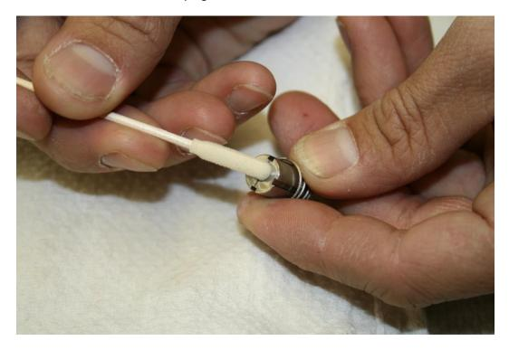
14. Insert the other end of the swab in the center of the plug and push the rubber stop and make sure it moves freely.
