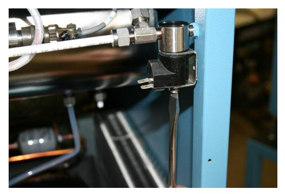
9. Remove the coil from the valve body.
