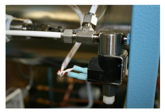
5. Take a 9/16" wrench and remove the bleed hose fitting at the bottom of the valve.
