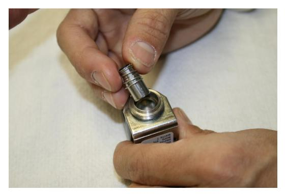
23. Place the o-ring over the center of the coil body.
