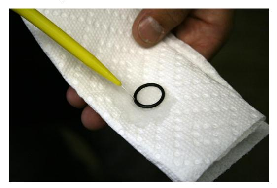
21. Apply a thin layer of valve lubricant/grease to the o-ring.
