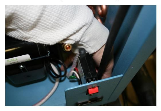
30. Replace the rear console panel and make sure to reconnect the fan power plug as well as the air in elbow and the main power cable on the rear panel.
