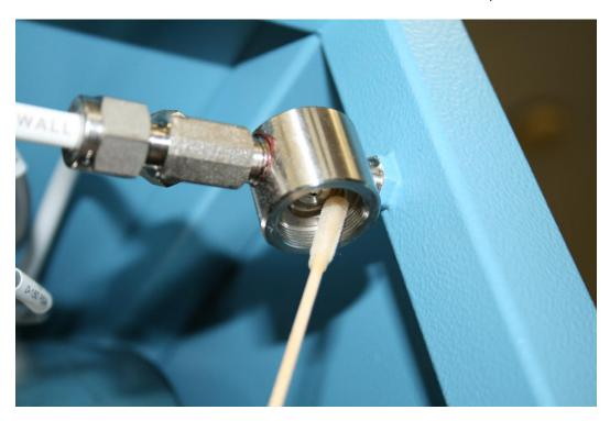
25. Align the coil body with the valve body and insert back into the valve body, taking care not to cross thread when screwing in the coil body.
