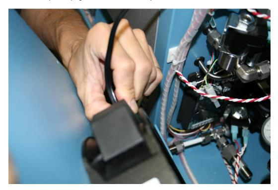
4. Locate the pressure bleed solenoid 3 at the top rear right hand corner of the system.
