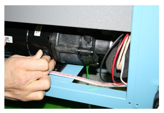
18. Once all the fluid has been drained carefully remove the pump.
