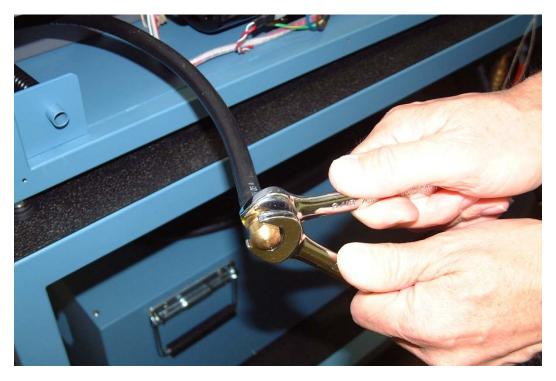
7. Release the fluid into a clean container large enough to hold approximately 3 US gallons, this fluid can be reused.
