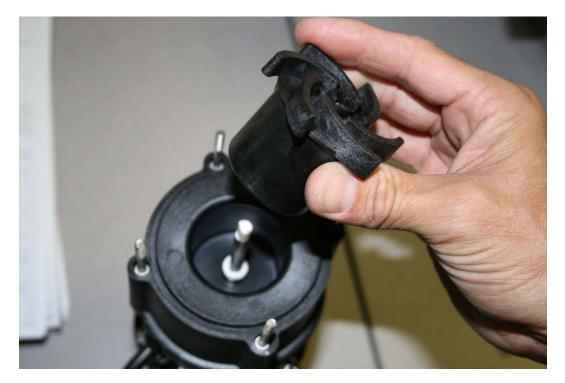
22. Remove the impeller shaft along with the thrust washer.
