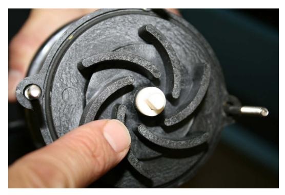
21. Remove the impeller/bushing from the impeller housing. Inspect and clean.
