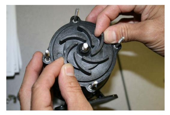
28. Align the key of the thrust washer with the shaft and push on.
