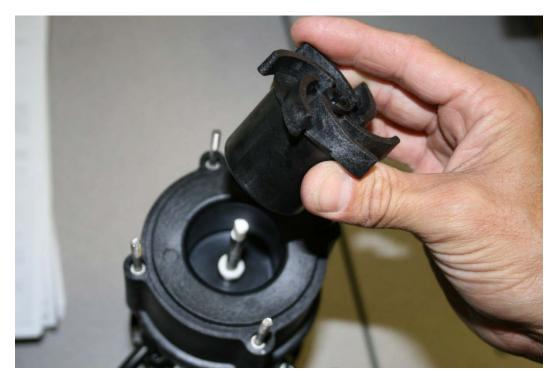
27. Carefully align the impeller/bushing in the center of the housing.
