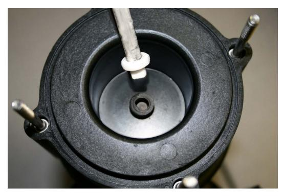
26. Slide the impeller/bushing over the shaft.
