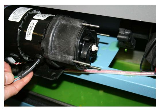
19. Inspect the o-ring for any debris, if any exists thoroughly clean.
