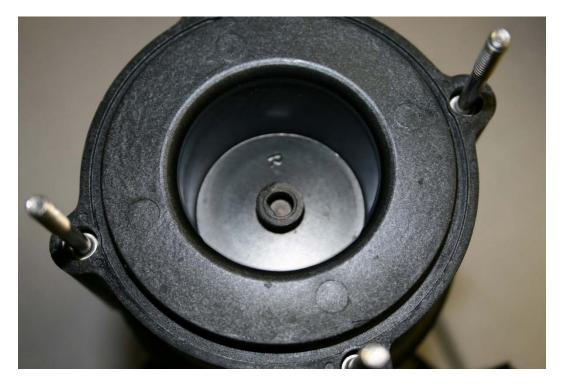
24. Clean the impeller shaft as well as the thrust washer, and then lubricate with non-drying silicone grease (Dow Corning #111 lubricant, recommendation).
