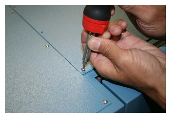
3. Remove the fluid fill port insulation plug.
