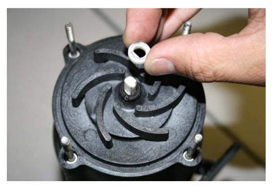
29. Slide the pump back in the system and make sure the o-ring is properly seated over the center of the impeller housing.
