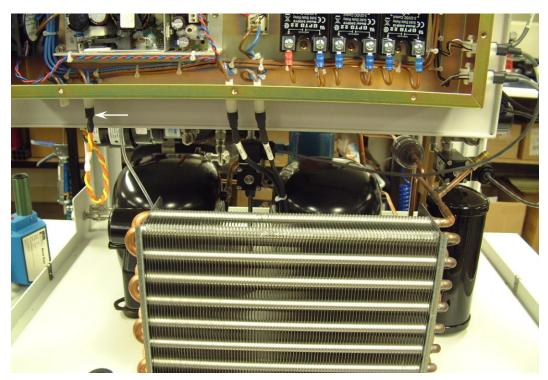
17. Route the power harness and plug it in to the electrical box as shown.
