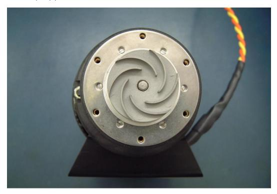
14. Carefully slide the motor into place and tighten the five screws. Use caution because the pump impeller is sharp enough to damage the Teflon seal.
