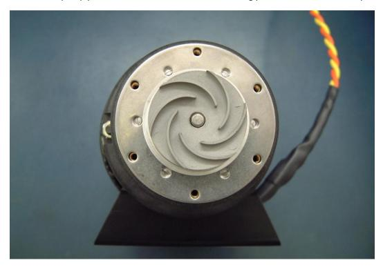
10. The impeller is magnetically coupled to the motor and will resist.
