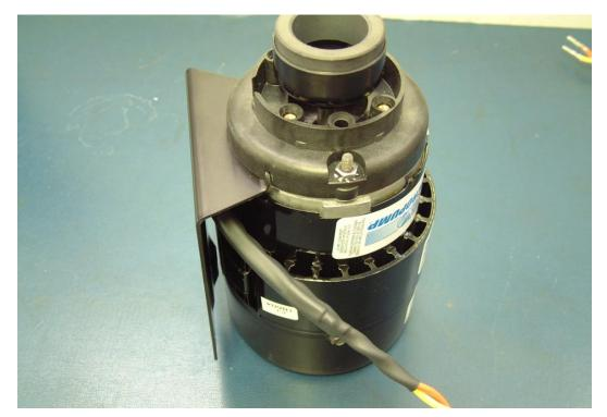
13. Place the pump parts back on the motor.
