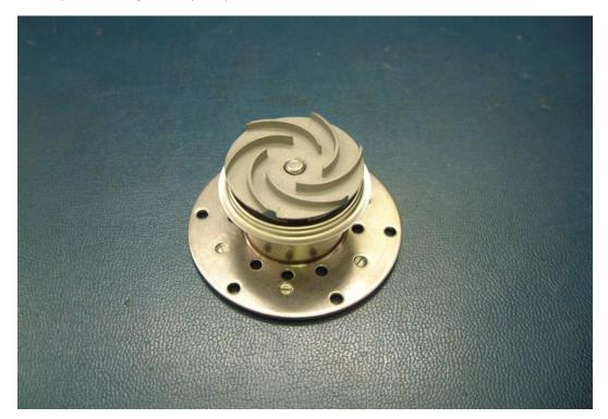
11. Use a 9/64" hex wrench to remove the two socket head cap screws from the motor adapter housing then remove housing. Remove any sealant from the housing. Do not damage the housing as it will be used on the new motor.
