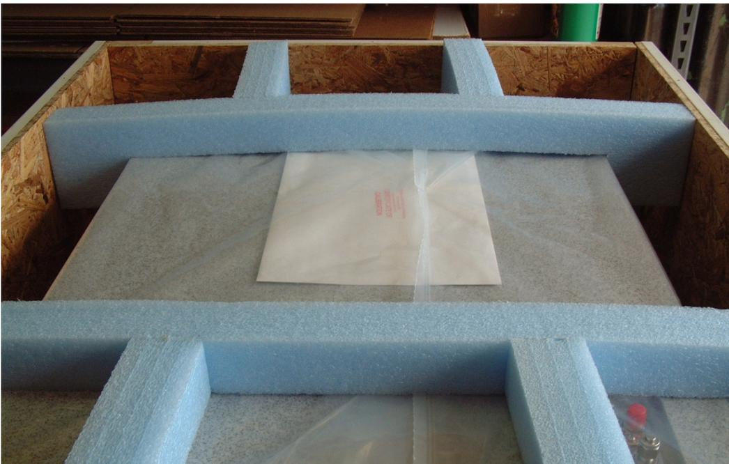
4. Insert the foam top pieces and slide the four foam corner braces in place.
