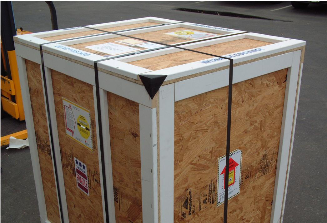
6. Put straps or steel banding around the crate in the locations shown so that the sides do not shift or separate from base. Two on the side support ribs and one across the front to back.
