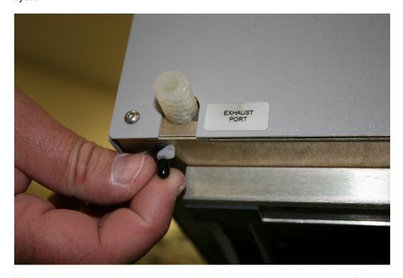
8. Replace the pressure vent cap, located underneath the system support rail at the rear right hand corner of the system.
