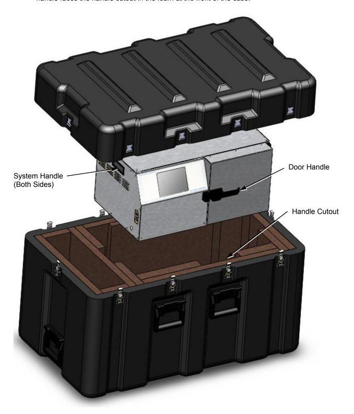
10. Put the case cover on and turn each case clasp until all are secured.
