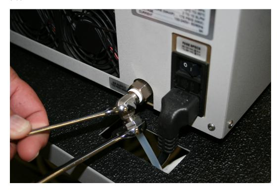
5. Remove the air in elbow using a 1/2" wrench and an 11/16" wrench as a backup.
