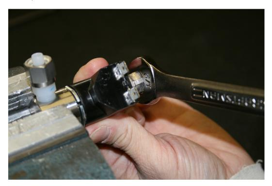
12. Turn out the solenoid component carefully.
