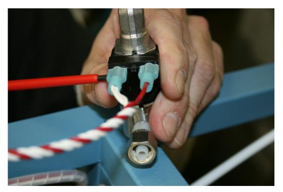
11. Take the valve to a work bench and place the stainless steel body in a vice. Using a 1/2" wrench, remove the elbow.
