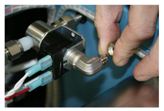
9. Pull back the other two nuts and remove the valve.
