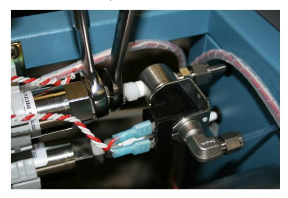
6. Next take a 1/2" wrench and use it as the backup wrench and use the 9/16" wrench to loosen the nut.
