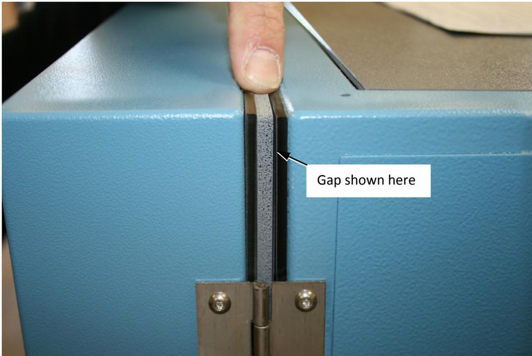
16. Open the door slightly once all the screws are in. Push on the bottom of the door at the hinge side of the door. This should push the door closer to the front chamber plastic panel and close up the gap.
