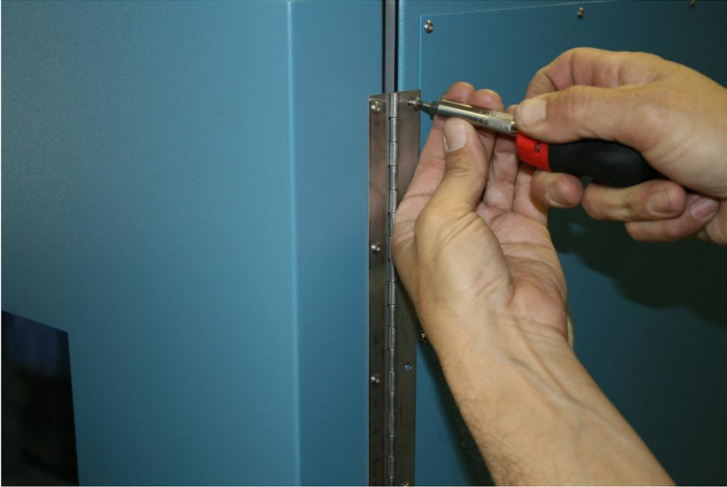
13. The next screw added will be at the bottom and leave it loose. Insert all the screws and snug up, all of them but allow some movement.
