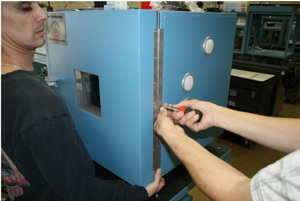
3. Peel off the old gasket and clean remaining residue with acetone and avoid painted surfaces. Wear gloves.
