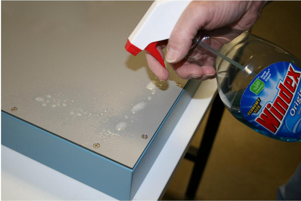
6. Working quickly; smear around the soapy water where the gasket will be.
