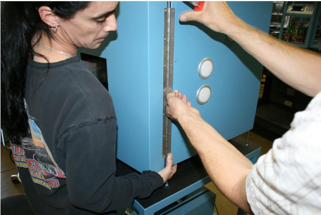
11. When installing the door, this is a two person operation due to the weight of the door, and installing the screws.
