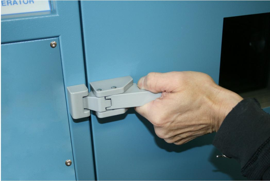
15. Look at the hinge end of the door to see if there is a gap between the gasket and the chamber plastic. Adjustment is needed in this case.
