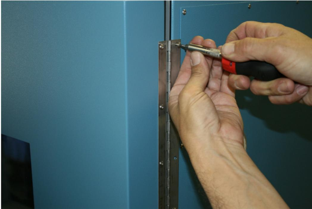
19. Shut the door and see if the latch has too much tension on it. Make sure the gasket gap and latch tension are all in a good state of balance.
