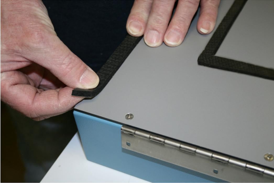
4. Lay the new gasket on flat surface with the paper side up and slowly peel paper the backing off.
