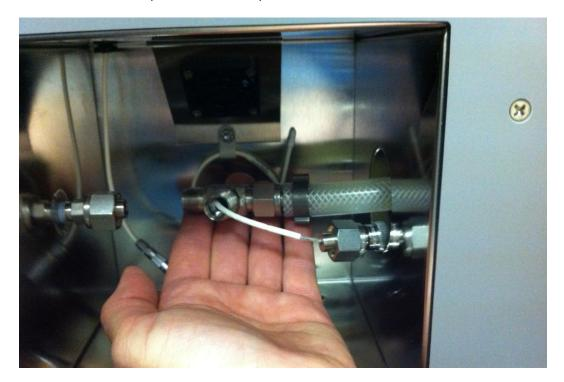
5. Connect the tee assembly to the fitting on 1200's inlet port. Reassemble the wire compression fitting to the tee assembly and tighten the knurled wire compression fitting just enough to keep the wire from sliding in the fitting. Align the red dots on connectors and push together.
