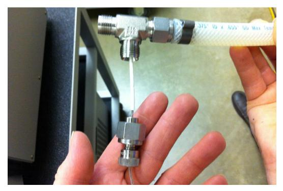
3. Insert assembly into access port as shown.
