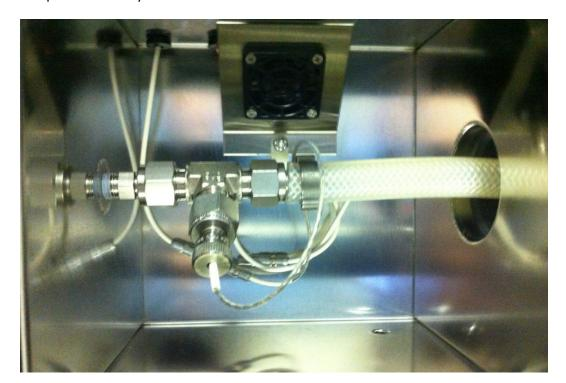
7. Remote calibration assembly, shown clamped to a humidity probe.
