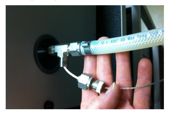
4. Make sure not to crimp the wires of the probe.
