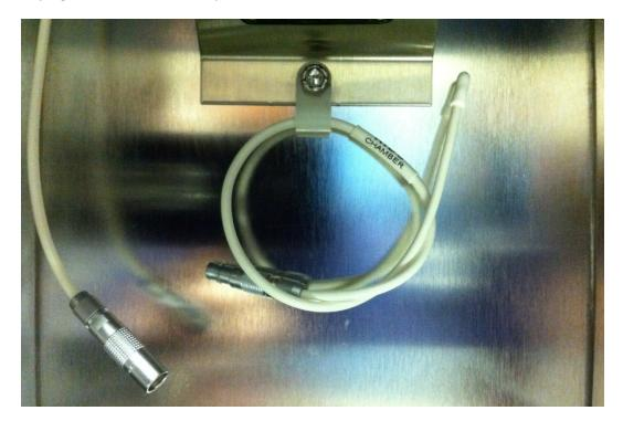
2. Loosen knurled wire compression fitting. Using an 11/16" wrench decouple the wire compression fitting from the tee.
