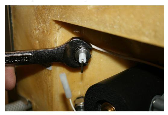
34. Remove the probe from the PreSaturator.
