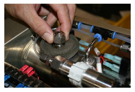
45. Using the 11/16" wrench tighten the reservoir fill port cap to 1/4 turn past finger tight.
