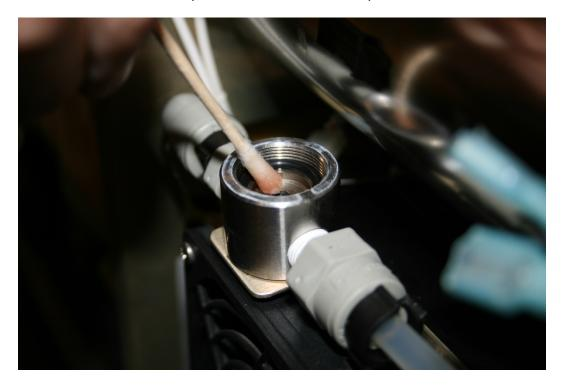
26. Put the coil back inside the stem and place it back in the valve body.
