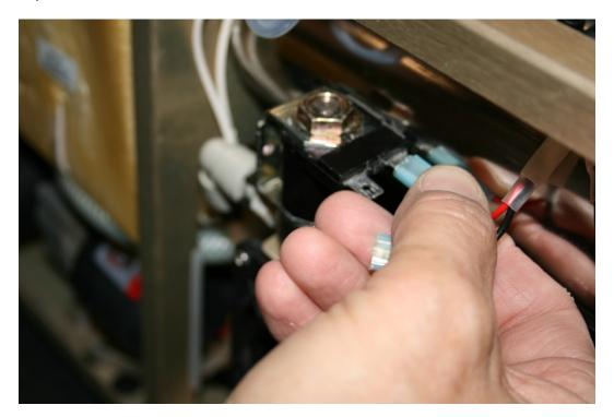
32. Next locate the liquid level probe (LL2) located on the side of the PreSaturator and pull the wire connector off.
