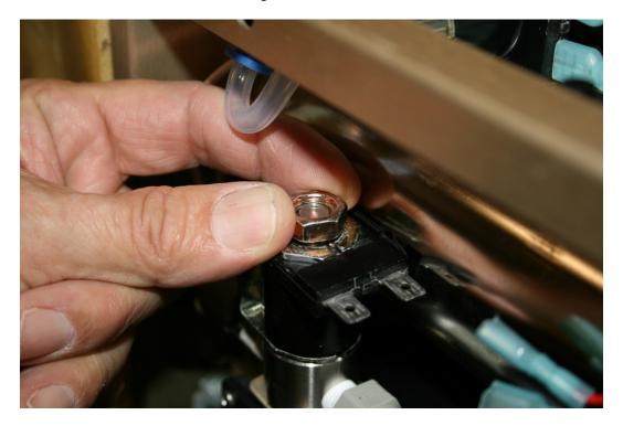
30. Tighten the nut down using the 9/16" open end wrench.
