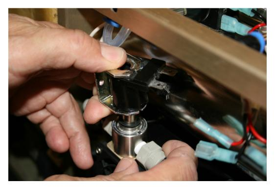
29. Put the nut back on the valve housing.
