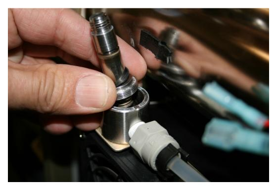
27. Tighten the stem back down using the channel lock pliers, turning clockwise until tight.
