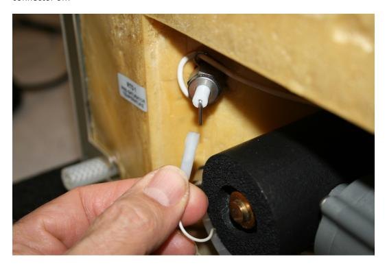
33. Using a 9/16" open end wrench, remove the probe nut.
