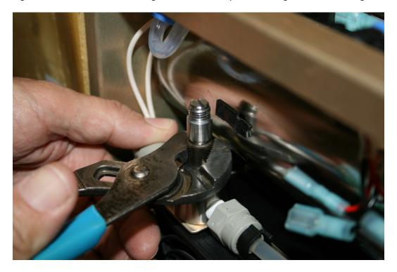
28. Replace the valve housing over the stem.
