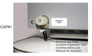
Location of the chamber overflow cap is the lower left hand corner.
