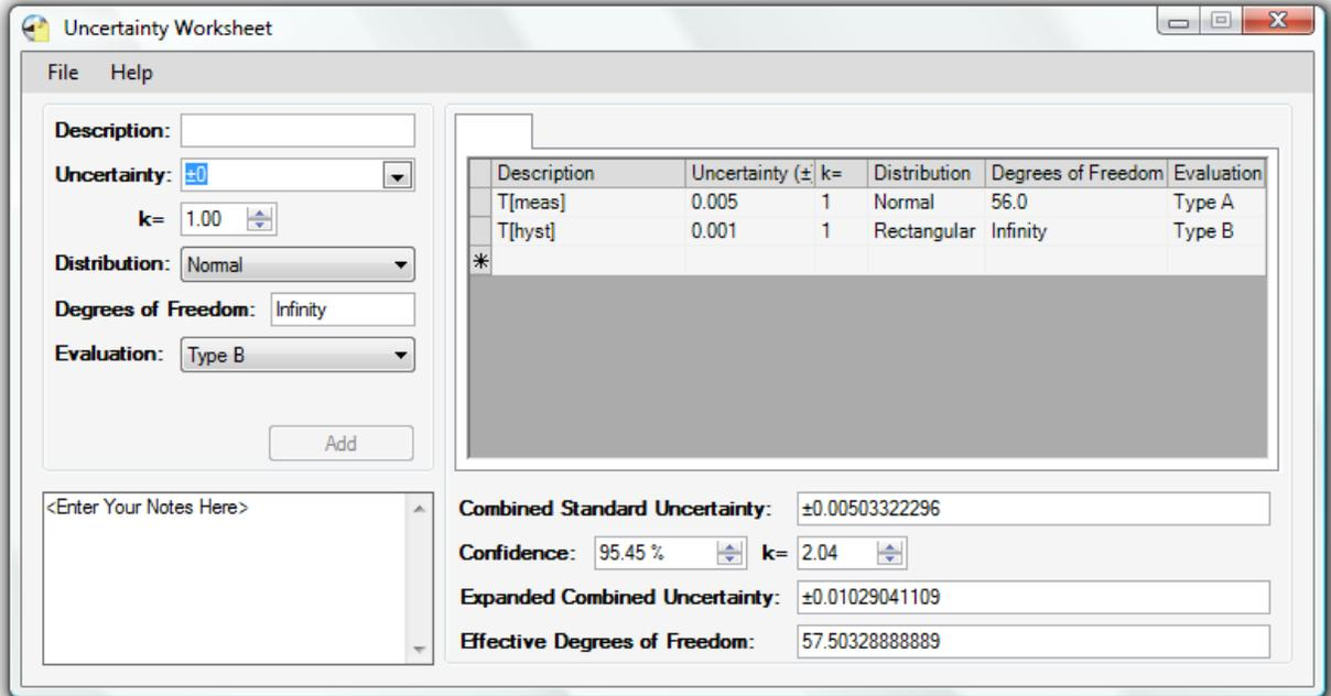
Last, enter the final individual uncertainty component values. The last component has a resolution type distribution and is again a Type B evaluation.
