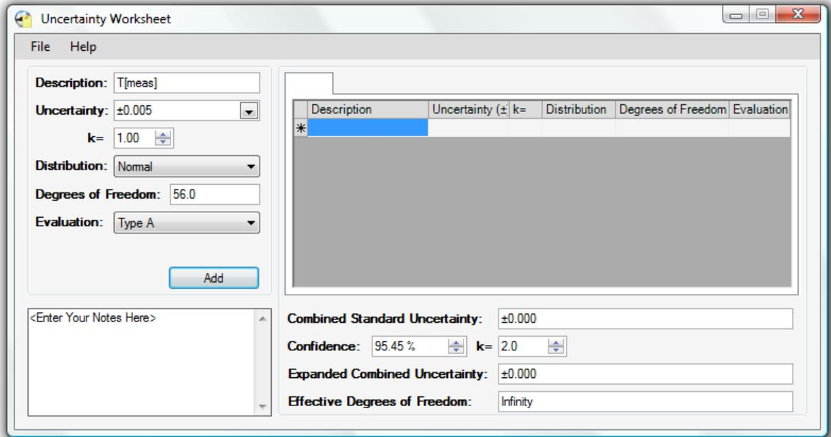
Once the information for the component has been entered, press the Add button to add the component to the worksheet.
