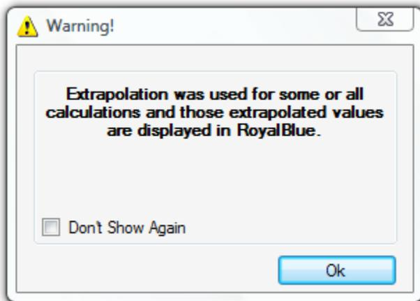
*\*Special Note on uncertainty and extrapolation: HumiCalc will not calculate any uncertainty if extrapolation was used in any part of the uncertainty calculation. This is simply because the uncertainty is unknown once outside the published limits of the humidity equations. Expanding the drop down uncertainty will result in the following drop down form message.*
