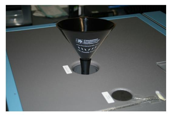
9. Using 2 U.S. gallons of 70% concentrate propylene glycol fluid, pour them in and fill the remainder with "recommended" distilled water until unit level is approximately 1/4" (6.35mm) below the bottom of the fill port.
