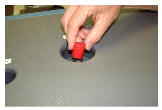
8. Use a funnel that will fit into a 5/8" (15.9mm) diameter opening, or use the one provided.
