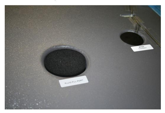
6. Remove the fluid fill port insulation plug.
