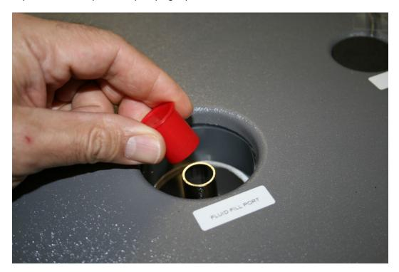
16. Insert the fluid fill port insulation plug.
