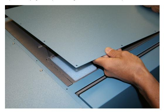
18. Replace the screws using your Torx screwdriver. Chamber fluid filling is now complete.
