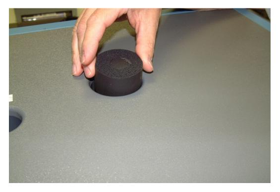
3. Remove the "Red" plastic fill port plug cap.
