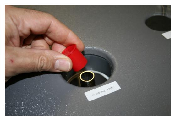
14. Put back the fluid fill port insulation.
