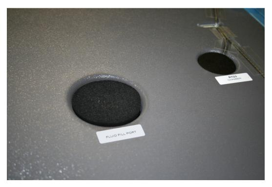
2. Remove the fluid fill port insulation plug.
