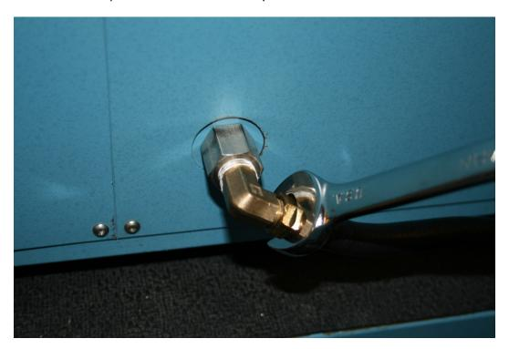
3. Next remove the air input elbow.
