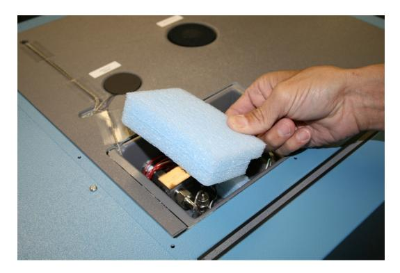
4. Remove the side expansion valve foam insulation.
