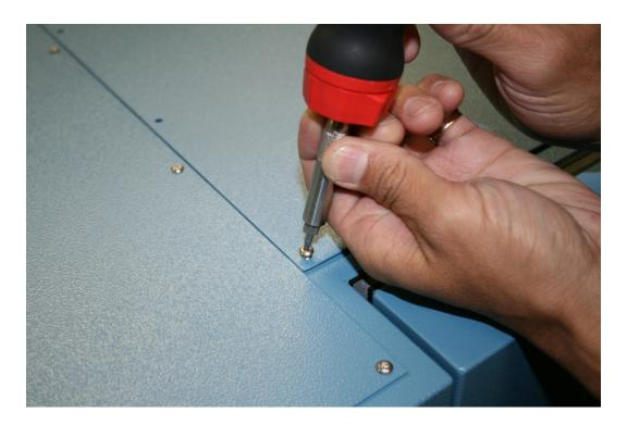
2. Using the Torx drive provided remove the Torx screws, and the right top panel.
