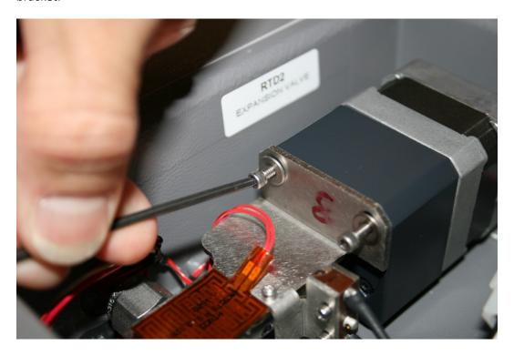
24. Only tightening the Allen screws to a loose fit.
