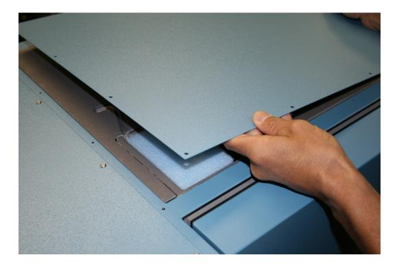
3. Remove the top expansion valve foam insulation.
