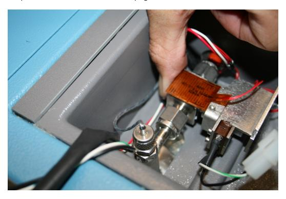
16. Before inserting the valve plug and gear assembly apply Krytox grease.
