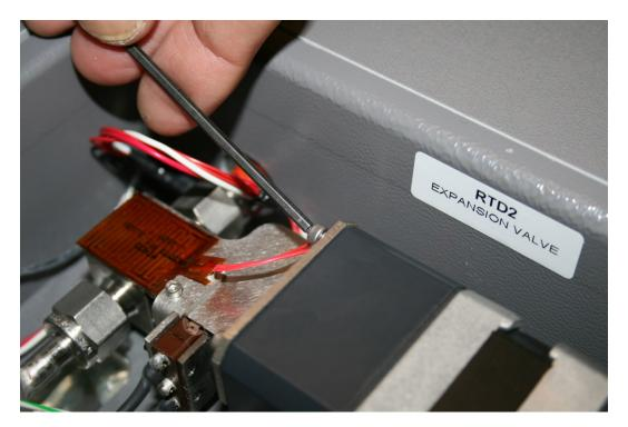
9. Rotate the valve motor 90° up to the vertical position.
