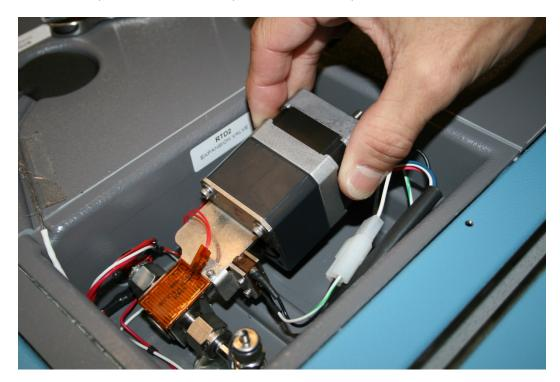
29. Turn on the main power switch and observe the Expansion valve coupling to notice if the roller switch lines up in the center of the valley of the coupling.
