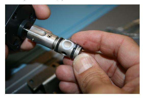
18. Before you put the value plug in place, make sure that the white Teflon O-ring is facing as shown, then move the roller switch out of the way and slowly push it into place carefully not to damage the Teflon O-ring at the top when inserted into the body.
