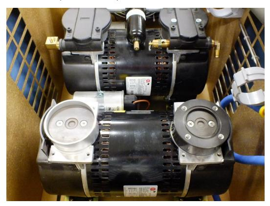
21. Torque retaining screws to 34-38 in.-lbs.
