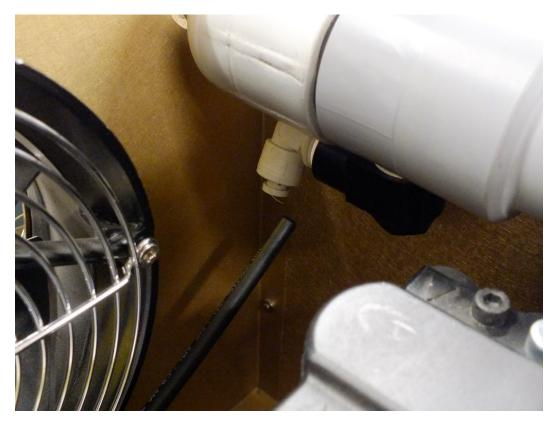
5. Unclip air dryer assembly and move out of the way.
