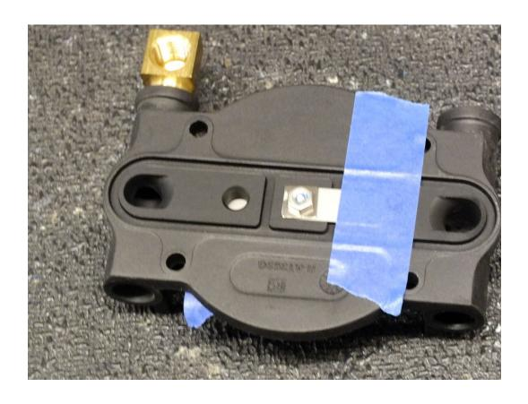
25. Clamp the valve plate in a vise and tighten screw.
