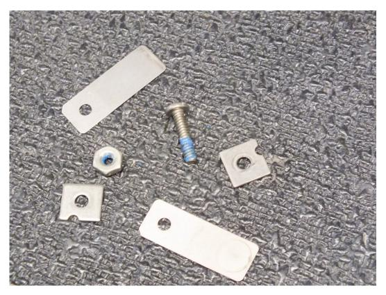
24. The valves are very fragile and should be handled with care. Note that the low-pressure valves are square on the end. Install new valves, retainer plates and screw onto the valve plate. The #6 nut may be re-used as a replacement but is not provided in the kit. Ensuring that the valves are oriented correctly, place a piece of tape over each valve so that they do not move while tightening the screw.
