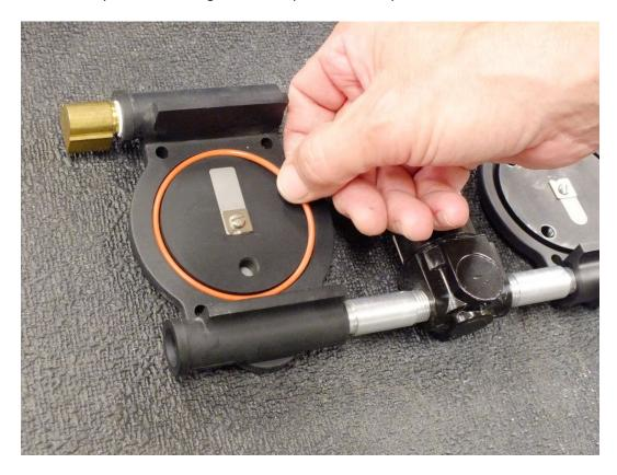
35. Carefully place the valve plates/filter assembly atop the cylinders.
