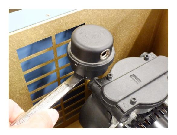
3. Disconnect swivel elbow from air dryer outlet by compressing lock ring and simultaneously pulling elbow.
