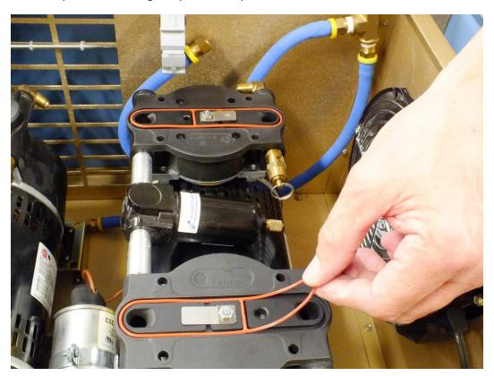
38. Install the valve covers, ensuring that they are oriented correctly.
