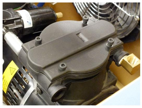
40. Torque all bolts to 50 in.-lbs. Re-install air dryer, hoses and filter.
