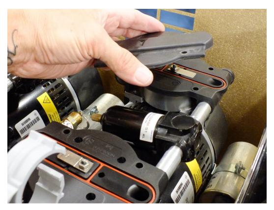
10. Remove the valve plates and filter assembly.
