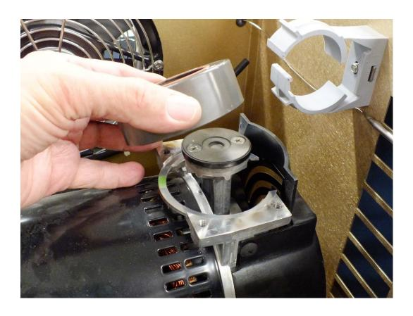
12. Using a #2 Phillips screwdriver, remove the screws from the high-pressure retainer plate and remove the retainer plates and piston cup.
