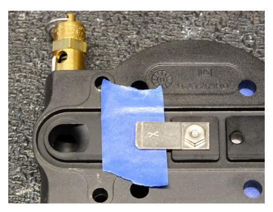
30. Tighten the screw and adjust the valve retainer and valve limiter if necessary.
