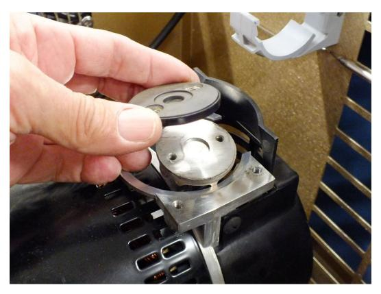
13. Note the orientation of the mark on the low-pressure retainer plate. Depending on the year model of the compressor, use either a T20 torx driver or 1/8" hex driver socket to remove the screws from the low-pressure retainer plate. Remove the retainer plate and piston cup.
