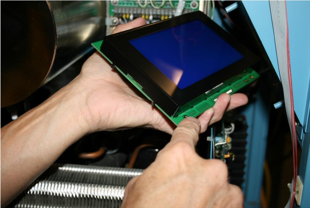
32. In the lower right-hand corner put the screw and washer on the bottom or back side of the display, then slide on only one washer over the screw on the front side.
