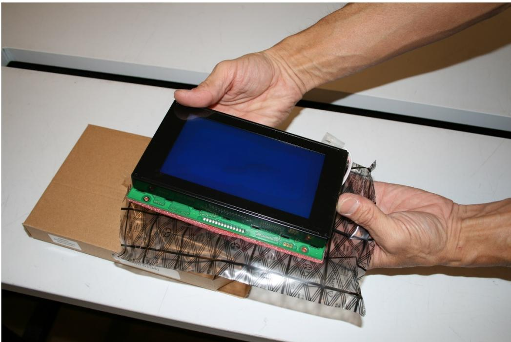
27. Remove the foam protection from the circuit board on the back.
