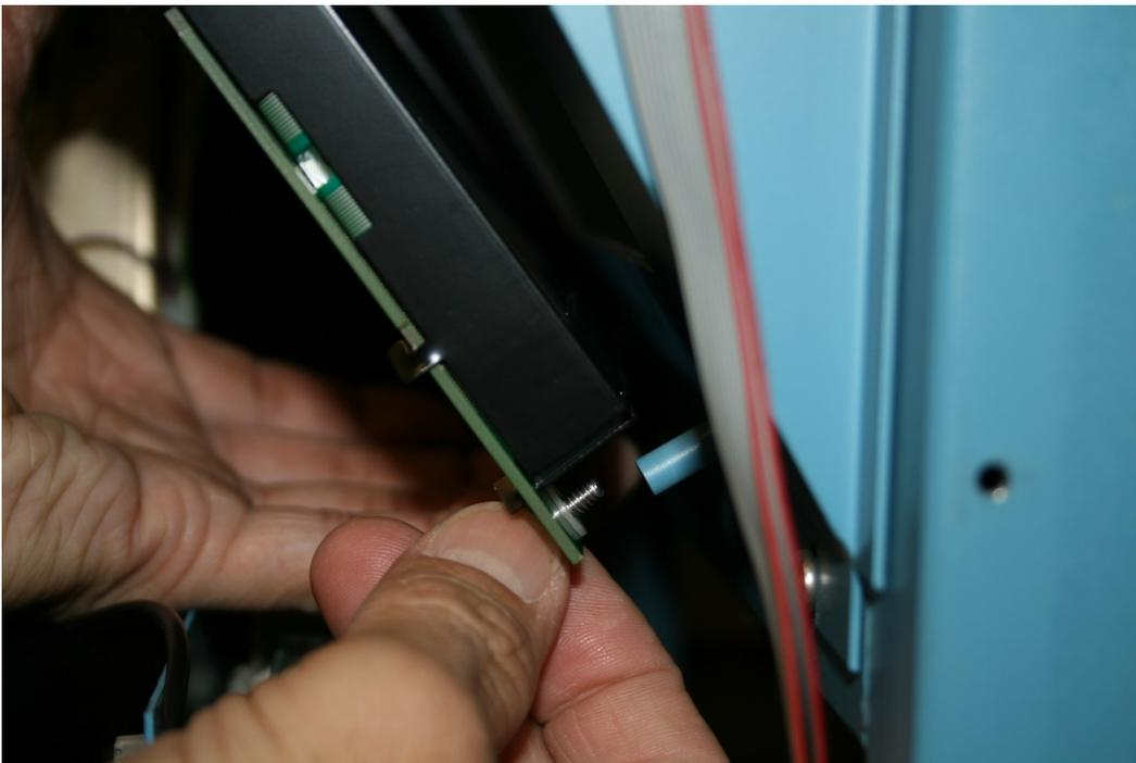
33. Twist in the screw in by hand so that it's just tight enough to hold the display in.
