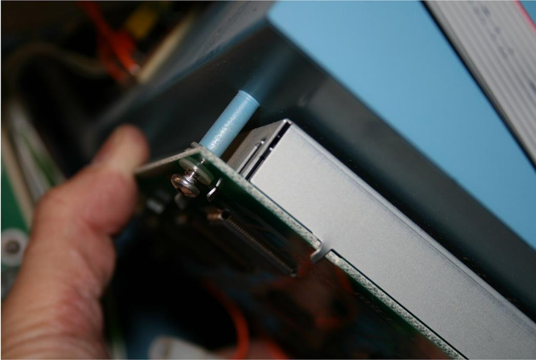
18. Carefully remove the top right-hand screw, and as you remove the screw grab the two nylon washers.
