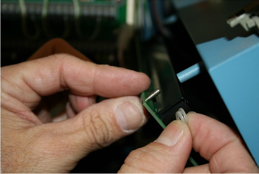
36. Screw it in by hand until it just catches the threads to hold the display up.
