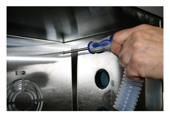
33. Reinstall the chamber temp probe and you are done.
