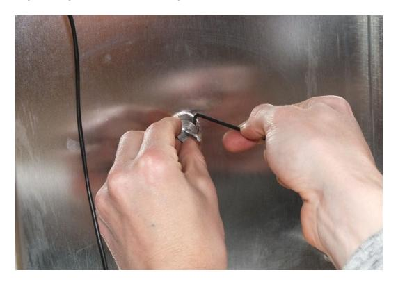
27. Push on the fan blade making sure the collar ring is towards the rear, and that the shaft sticks out by 1/4".
