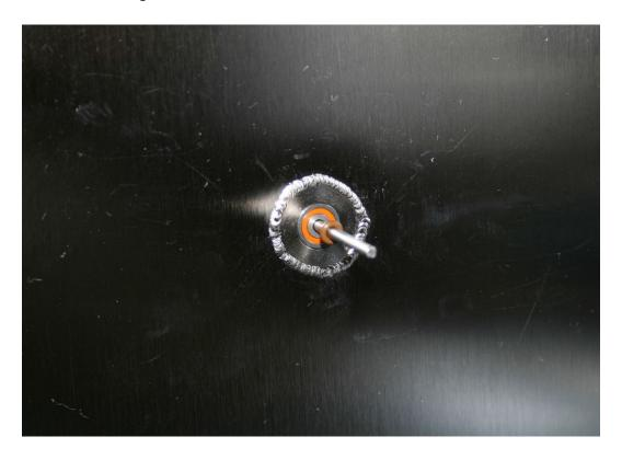
25. Apply Krytox 240AB grease to the O-Ring and smooth side of the Shaft Collar.
