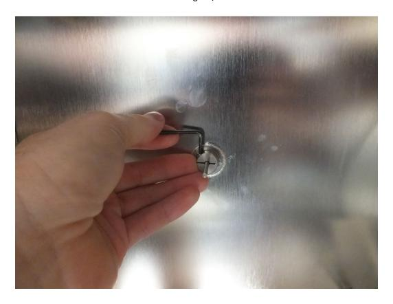
14. Move to the rear of the unit and use a 6/32" Allen wrench, remove the three #6-32 x 3/8" Socket Head Cap Screws at the fan motor assembly.
