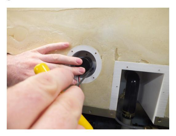
31. Reinstall the fan shroud but first make sure the standoffs are tight first.
