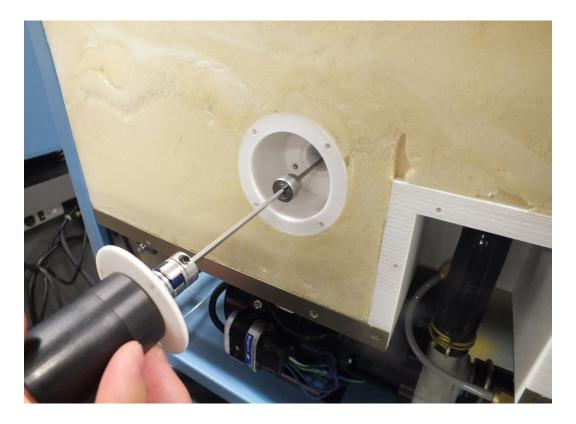
17. Manipulate the shaft and guide the Bearing into outer race and pull the shaft, make sure it seats fully. Then pull on the shaft.
