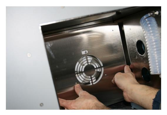
32. Using a Phillips head screwdriver, use the same four #8-32 x 1/4" Pan Head Phillips head screws to mount the panel.
