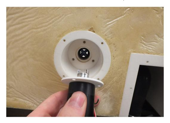
16. Take the new shaft assembly and place it on the fan motor Jaw Coupling Hub and slide it into the motor housing tube and replace the three  $\#6-32 \times 3/8$ " Socket Head Cap Screws.
