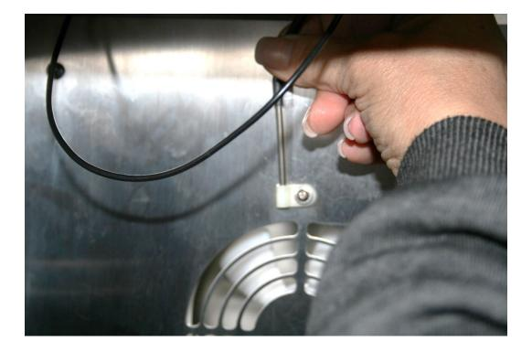
11. Remove the fan shroud panel using a Phillips head screwdriver and save the four  $\#8-32 \times 1/4$ " Pan Head Phillips head screws.
