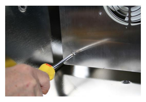
12. Take off the fan using a 1.5mm Allen wrench and remove the set screw collar and take note which way the fan is facing. If it's an older model, then just pull the fan off.
