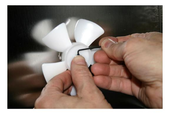
30. Reinstall the fan motor assembly using the three  $\#6-32 \times 3/8$ " Socket Head Cap Screws to secure it.
