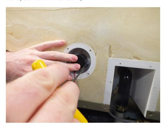
15. Pull out the fan motor assembly and if it doesn't come out with the shaft you will have to push the shaft from the inside of the chamber and do not use old shaft parts.
