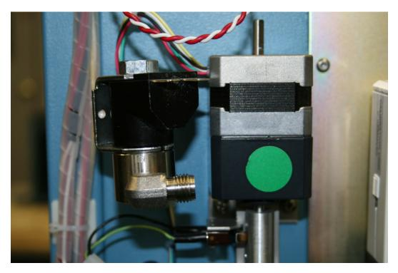
25. Reattach the reservoir to pre-sat solenoid tube using a 9/16 wrench and a 1/2 wrench, be sure not to over tighten.
