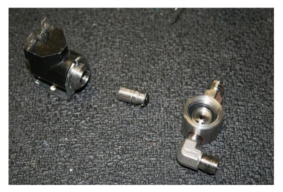
12. Remove the o-ring from the valve body.
