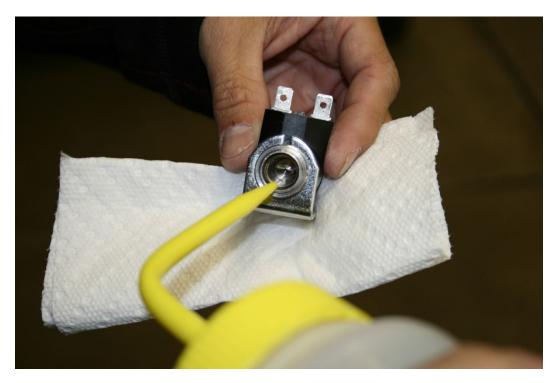
18. Use a swab to get any debris from inside the coil chamber.
