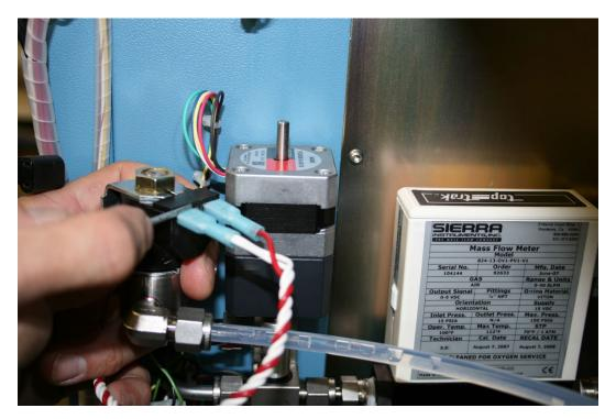
5. Loosen the nut on the elbow of the reservoir to pre-sat solenoid tube.
