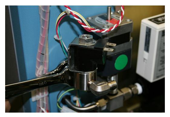
24. Make sure that the elbow is level with the frame.
