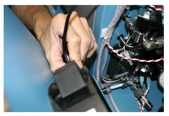
4. Locate the Pre-Sat fill solenoid and remove the wire leads using a small flat head screwdriver.
