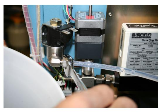
6. Make sure you have a one gallon bucket in close proximity to the tube nut and move it over to the bucket to let the reservoir drain.
