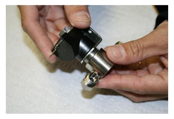
22. Make sure that when you assemble the two parts the coil needs to be at a 45° angle towards the elbow before tightening it down.
