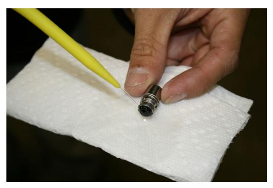
15. Clean the valve body with alcohol.
