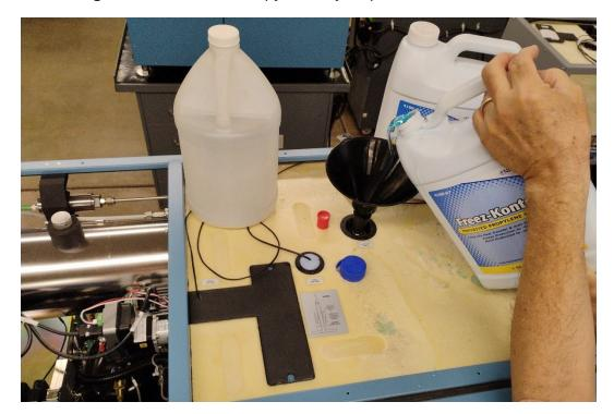
8. Then continue to fill the remainder with water until the level is approximately 2" below the top of the fill port. See Chamber Cut-A-Way on next page.
