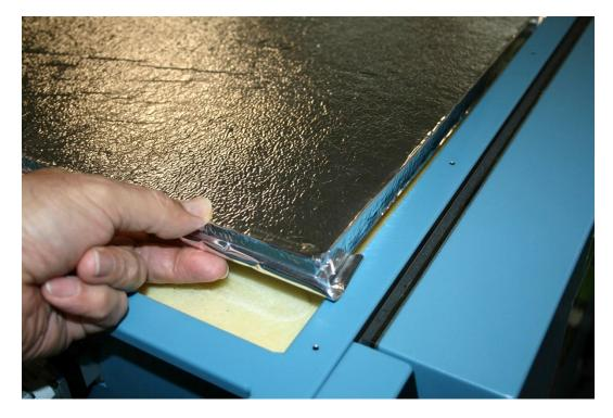
16. Install the top console panel and tighten the Torx screws that were removed from the previous steps.
