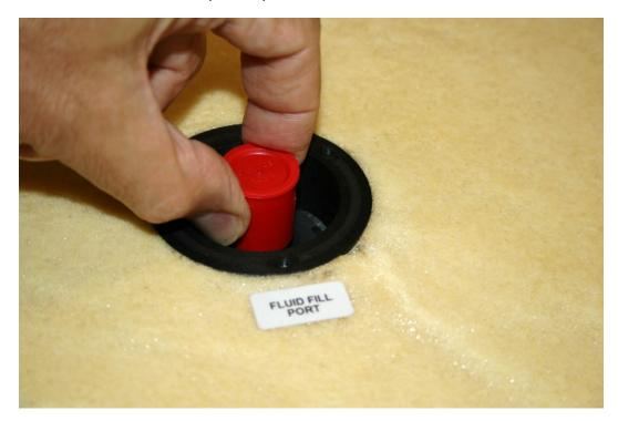
6. Insert the Chamber Fill Funnel into the Fluid Fill Port.
