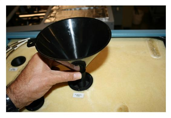
7. Add 2 gallons of Inhibited Propylene Glycol provided with model 2900.
