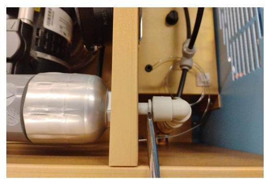
7. Then pull the elbow away from the Membrane Air Dryer.
