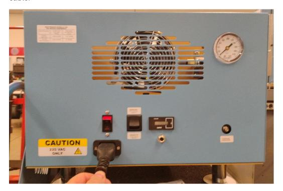
2. Remove the Air Outlet Hose using a 9/16" wrench on the hose and an adjustable wrench on the Air Outlet Elbow.
