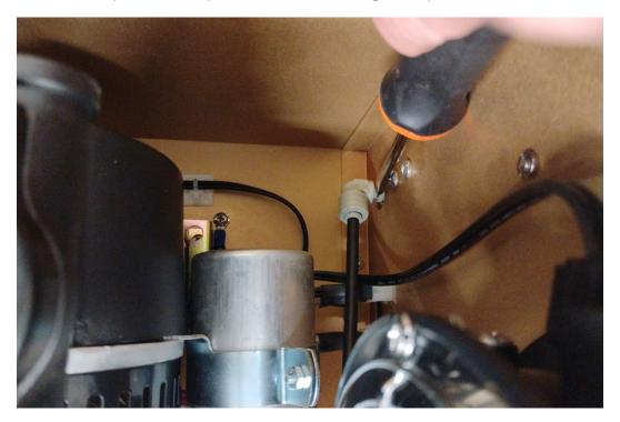
14. Remove the elbow and tube from the ACS2520 and discard these parts.
