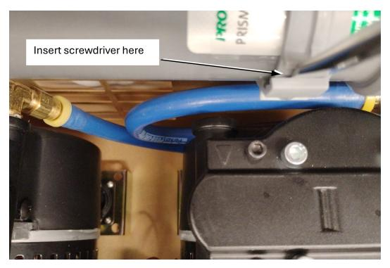
9. Remove the black tubing located on the underside of the Air Dryer. Use a flat head screwdriver to push in the quick disconnect fitting, then pull the tube out.
