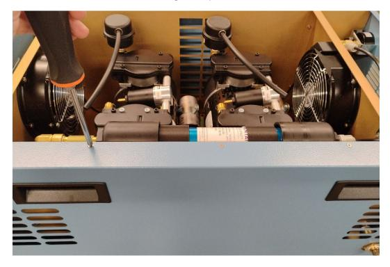
32. Reinstall the eight  $\#6-32 \times 1/4$ " pan head screws along the side.
