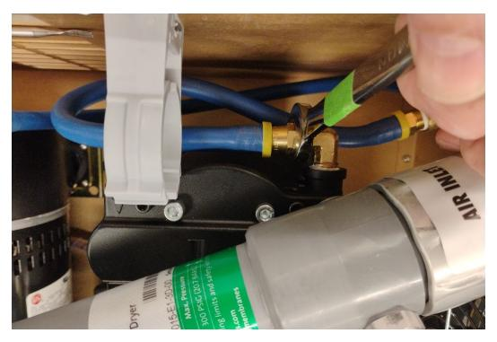
13. Remove the elbow located on the back side of the regulator. Using a flat head screwdriver, push in the quick disconnect fitting, then pull the tube elbow out.
