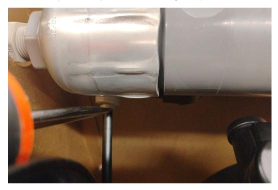
10. Remove the Air Dryer by pushing it as far to the right as possible while simultaneously pushing the compressor to the right, providing room for the fitting underneath to clear. See the next photo for compressor clearance.
