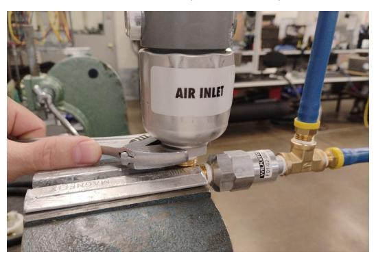
19. Remove the Inline Particulate Filter from the elbow and discard the elbow.
