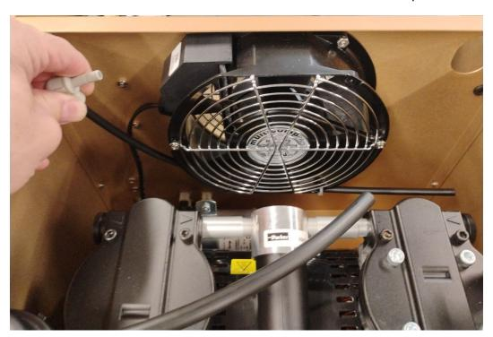
15. Replace the elbow with the push in muffler provided with the kit.
